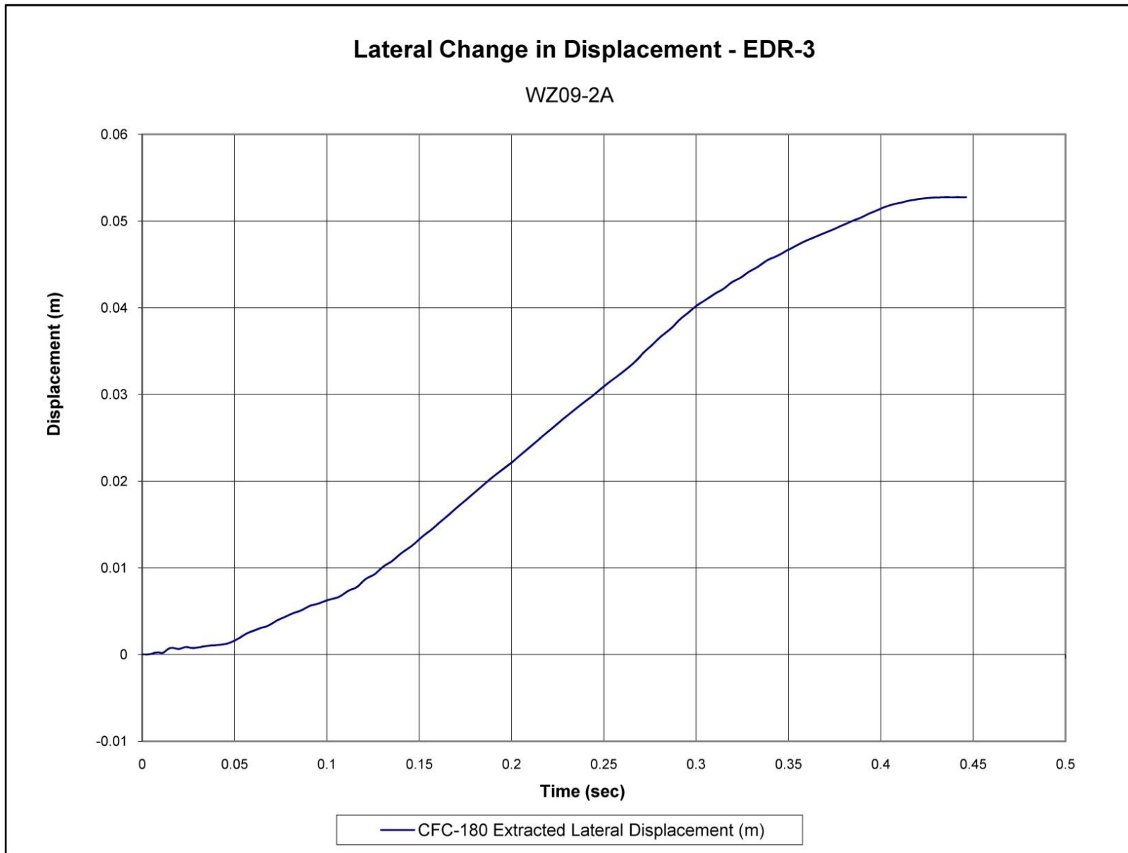
Figure G-6. Lateral Occupant Displacement (EDR-3), Test No. WZ09-2A
