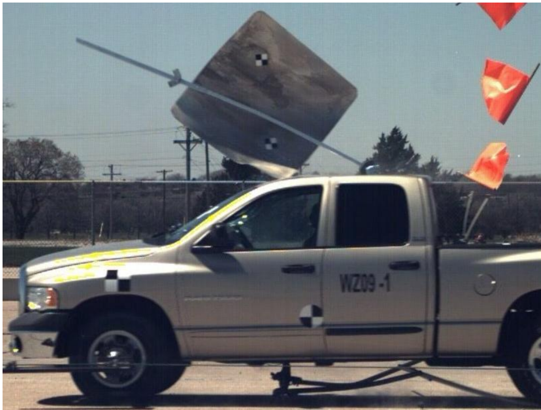
Figure 106. System No. 1A, Flag Holder Penetrating the Roof
