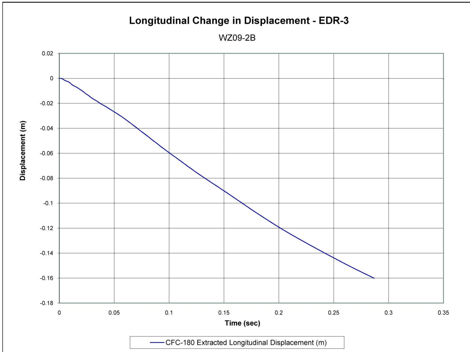
Figure G-16. Longitudinal Occupant Displacement (EDR-3), Test No. WZ09-2B
