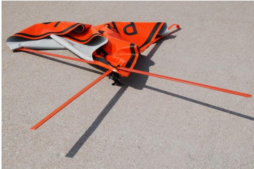
Figure 96. System Damage, Test No. WZ09-4A
