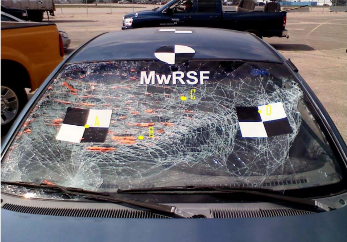
Figure E-7. Windshield Deformation Data, Test No. WZ09-3
