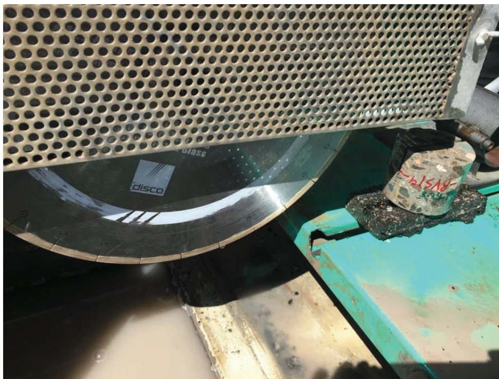
Figure 2.7: J-slot continuous diamond blades for concrete core cutting.
