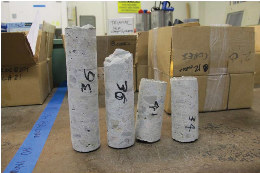
Figure 2.2: Bridge cores; cores equal to or longer than 3 inches were used for ASR visual inspection.
