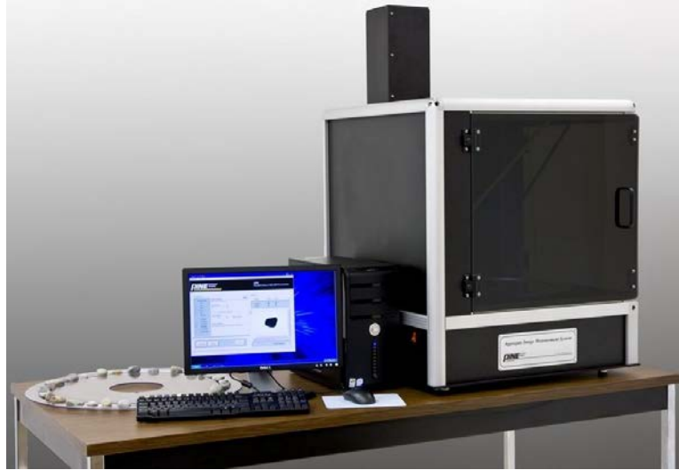
Figure 1.1. Second generation Aggregate Imaging Measurement System (AIMS-II).
