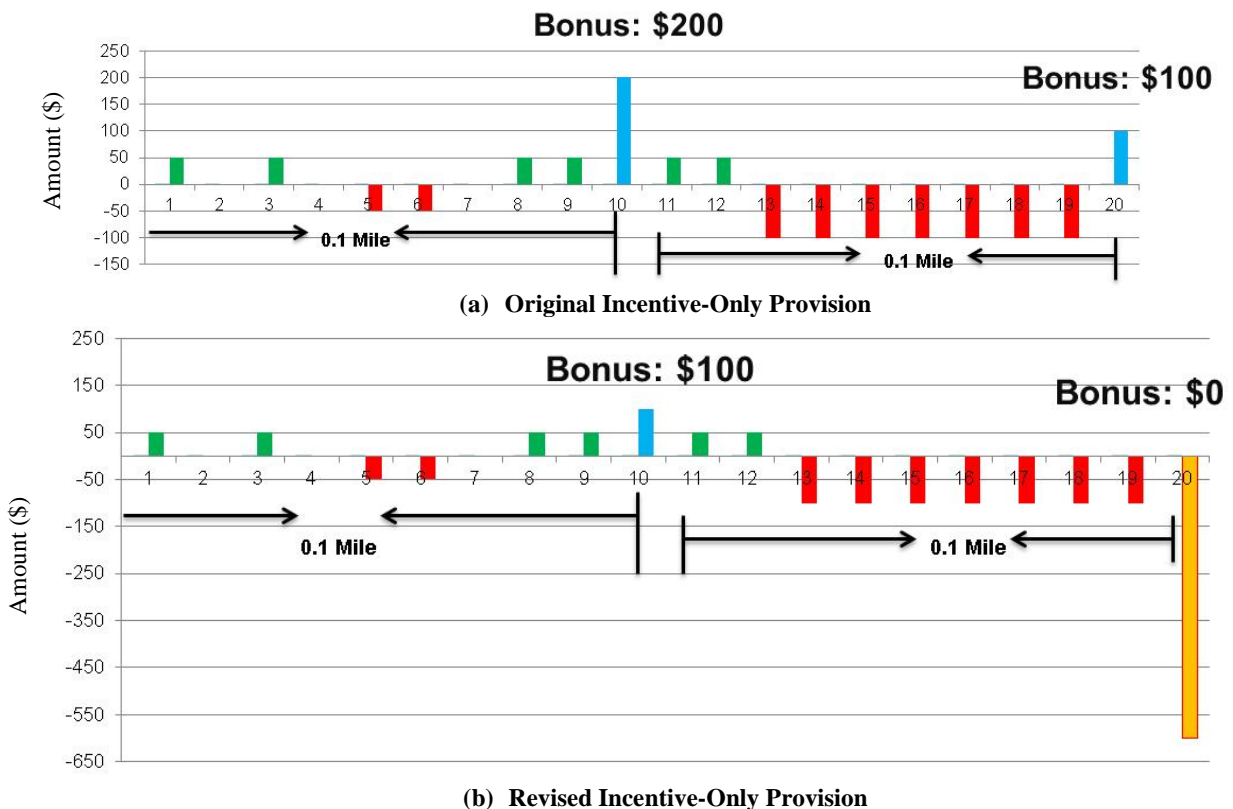
Figure 1. Example Framework for Incentive-Only Pay Adjustments. Green bars = incentive; red bars = disincentive.
