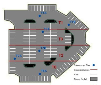
Figure 2. Diagram of the Porous Asphalt Park & Ride Facility Showing Different Maintenance Sections and Sampling Locations
