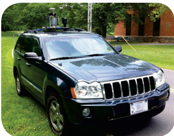
Figure 10. Photo. Vehicle equipped with sensor platform on roof.
