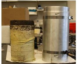
(a) Compacted 150 mm diameter sample
