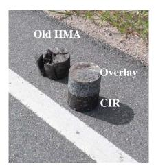
Figure 83. Cored Asphalt Samples from the SH 86 Kiowa East
