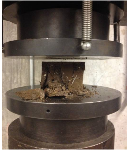
Figure 3.3 Completed USC test on Type II CEAM.
