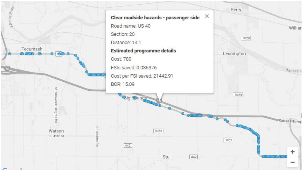
Figure 5.6: Countermeasure Information at a Selected Segment along US-40
