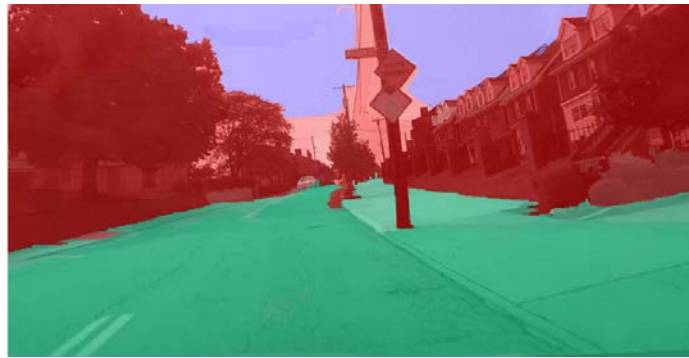
Figure 7 Image segmented into ground plane (green), objects (red) and sky (blue).
