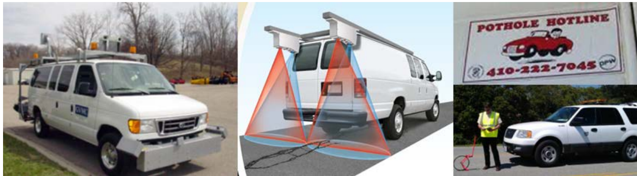
Figure 1 Methods of road inspection: Camera based 3 (left) and laser based 4 (middle) specialized vehicles, hotline (right top) and road inspector (right bottom).
