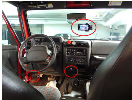
Figure 2 Smartphone mounted inside a vehicle. It is powered by the cigarette lighter. An OBDII-to-Bluetooth device is installed under the dashboard.
