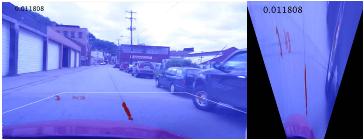
Figure 11 The area in front of the vehicle (outlined with a white line in the left image) is projected into a bird's eye view (right). The distress score is the area with cracks (red) divided by the total area. In this case the distress score is 0.012.
