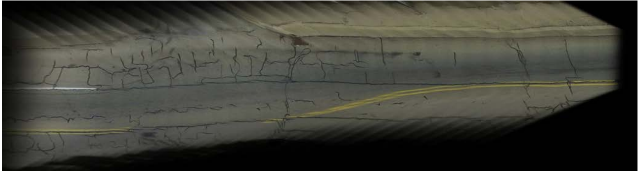
Figure 12 A bird's-eye-view of a road stitched together from about 60 images.
