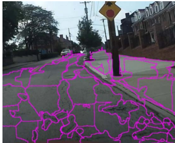
Figure 8 The ground plane segmented into superpixels.
