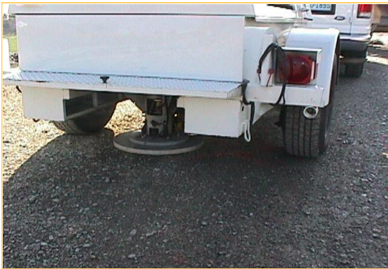
(a) FWD testing using a circular plate
