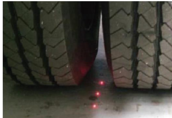
(b) TSD measuring deflection velocity between the dual tires
