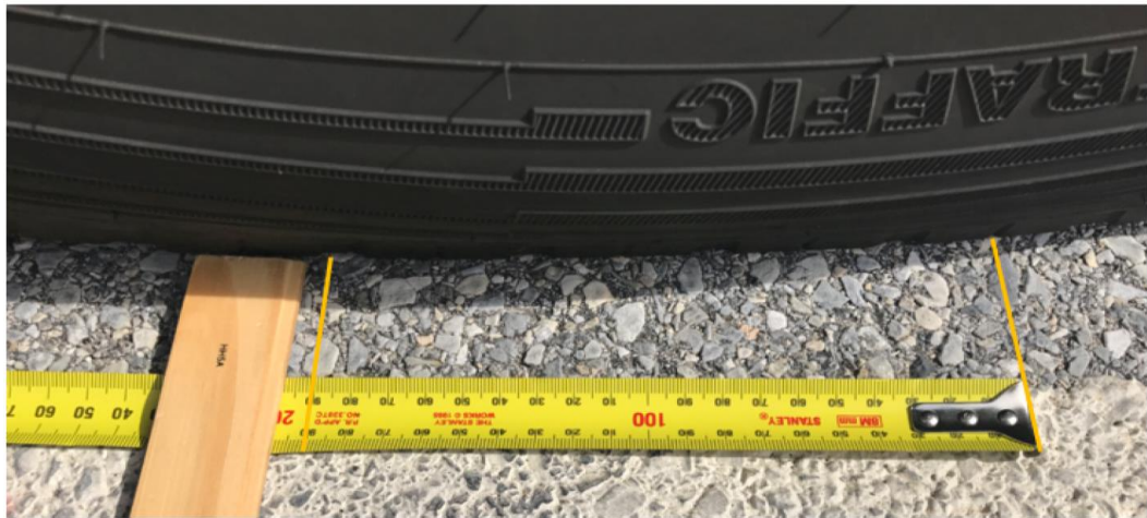
(b)TSD tire dimensions in longitudinal (traffic) direction
