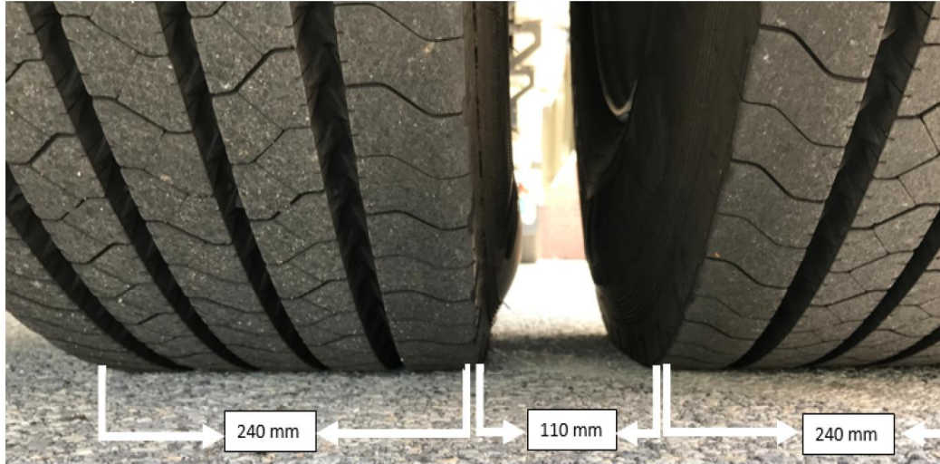
(a)TSD tire dimensions in transverse direction
