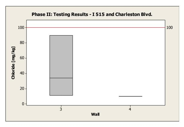
Figure 3-16: Phase II chloride results for I-515 and Charleston Blvd., separated by wall
