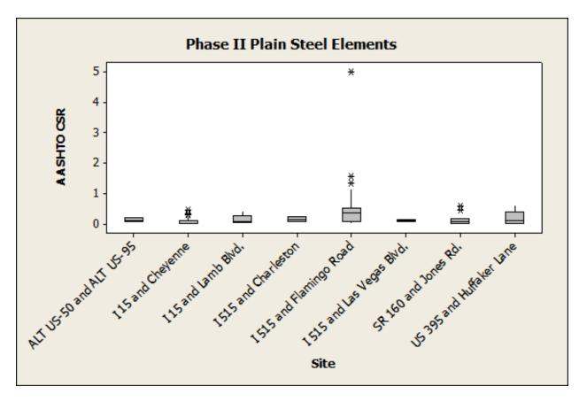
Figure 4-34: Phase II plain steel coupon AASHTO corrosion severity ratios based on site wide information, I-515/Flamingo Rd. included as reference
