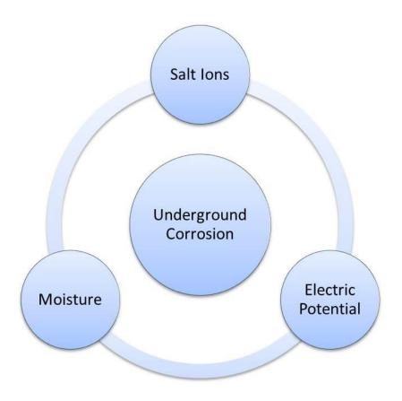
Figure 2-1: Underground corrosion interdependency
