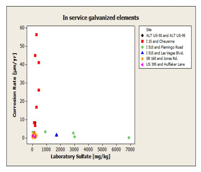
Figure 4-5: LPR corrosion rates compared to the sulfate content, full spectrum of Phase II data
