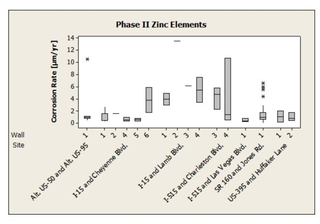
Figure 4-23: Phase II zinc elements corrosion box-plots, per wall distribution of LPR corrosion data
