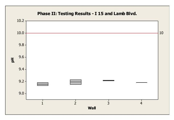
Figure 3-14: Phase II pH results for I-15 and Lamb Blvd., separated by wall
