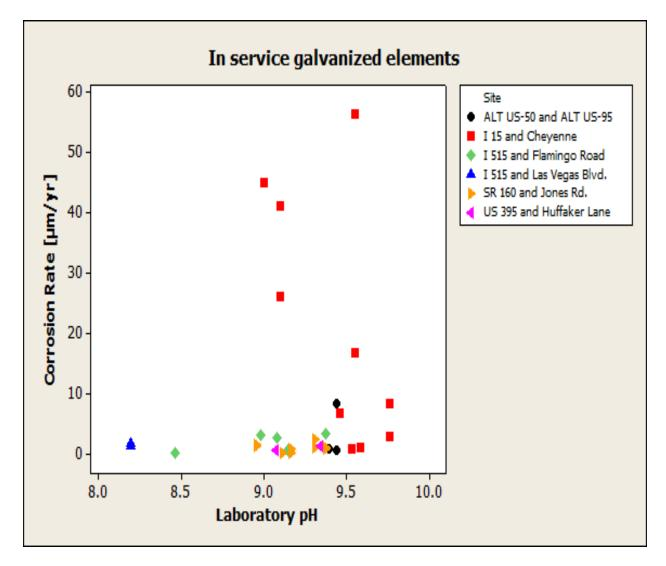
Figure 4-11: Phase II LPR corrosion rate data compared with backfill pH test results
