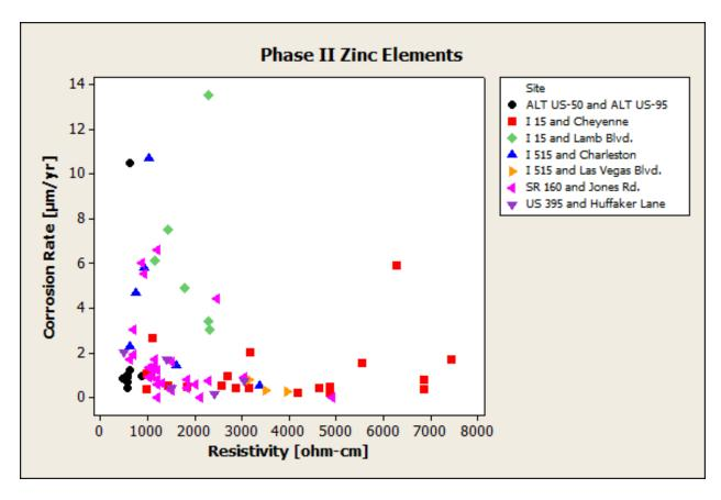
Figure 4-19: Phase II Zinc element LPR corrosion rates compared to the complete minimum soil resistivity testing results
