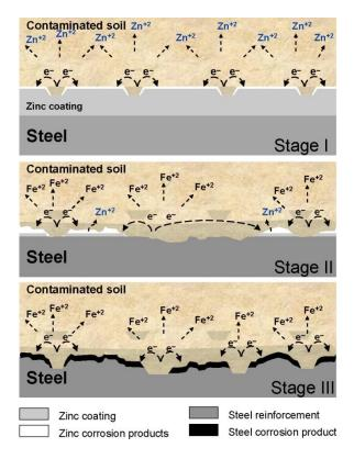
Figure 2-3: Schematic showing the three phases of galvanic corrosion (Padilla et. al. 2013)
