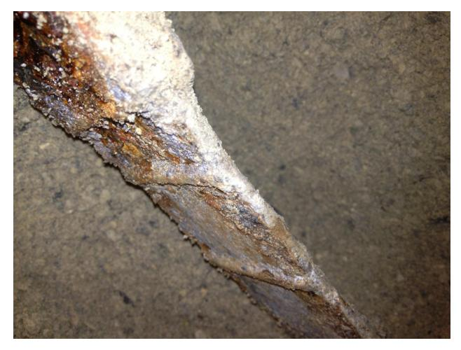
Figure 5-16: In-service galvanized soil reinforcement for I-15/ Cheyenne Blvd. Wall 1, 15 years old.
