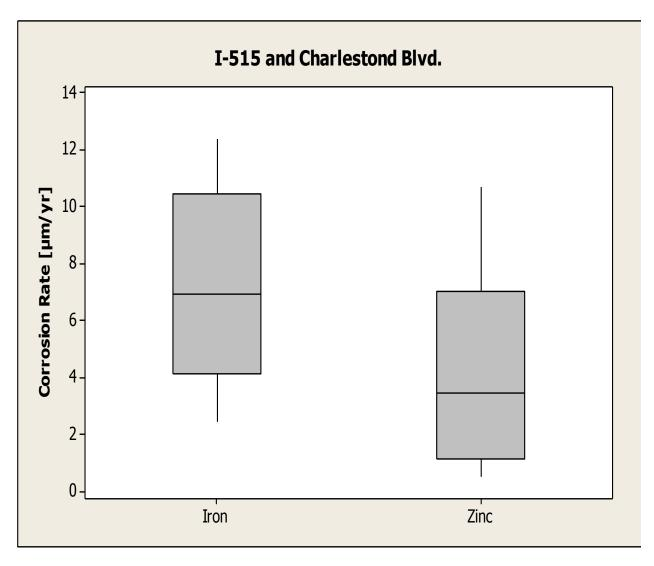
Figure 5-21: Phase II LPR corrosion rate box-plots by element type for I-515/ Charleston Blvd.
