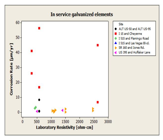
Figure 4-10: Phase II LPR corrosion rate data in soils that FAILS the 3,000 ohm-cm specification for minimum soil resistivity
