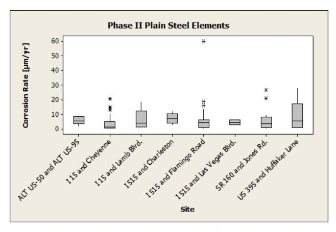
Figure 4-33: Phase II plain steel LPR corrosion rates grouped by site, I-515/Flamingo Rd. included as reference
