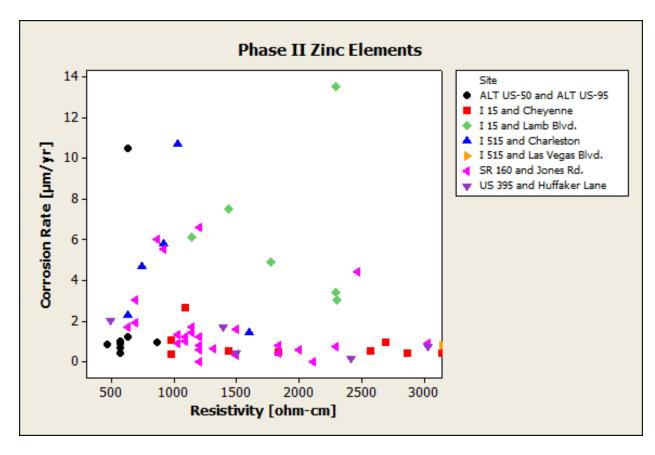
Figure 4-20: Phase II Zinc element LPR corrosion rates for elements in backfills that fail specifications for minimum soil resistivity
