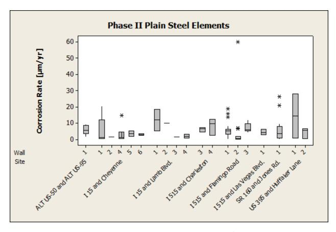
Figure 4-32: Wall specific LPR corrosion rates of Phase II plain steel coupons data, I-515/Flamingo Rd. included as reference
