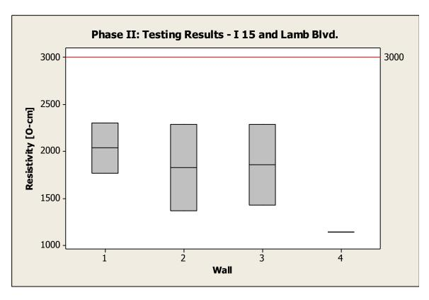
Figure 3-13: Phase II resistivity results for I-15 and Lamb Blvd., separated by wall
