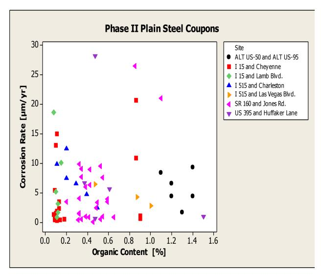
Figure 4-31: Phase II plain steel coupon LPR corrosion rates with respect to organic content of MSE wall backfill
