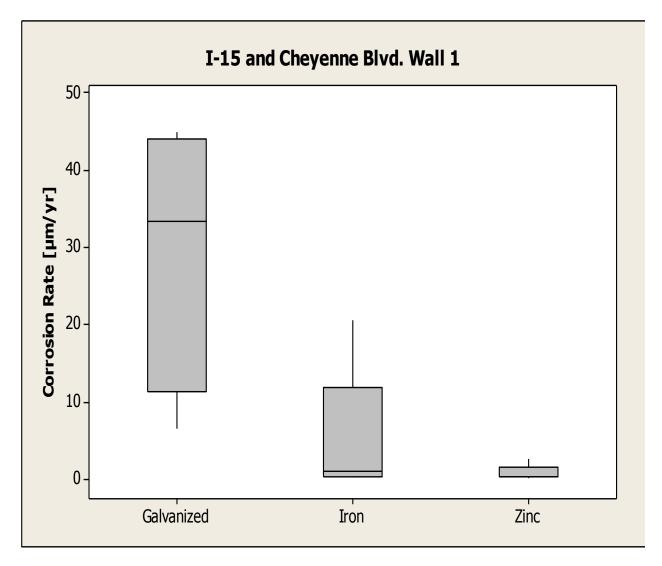
Figure 5-11: Phase II LPR corrosion rate box-plots by element type for I-15/ Cheyenne Blvd. Wall 1
