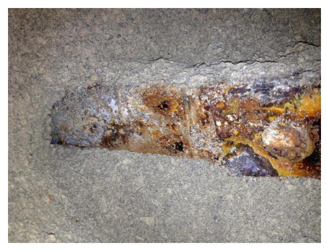
Figure 5-13: In-service galvanized soil reinforcement for I-15/ Cheyenne Blvd. Wall 1, 15 years old.
