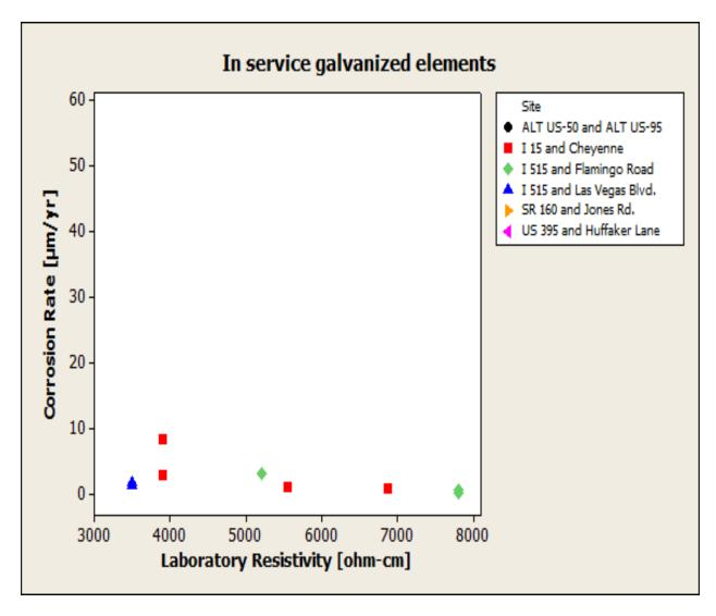
Figure 4-9: Phase II LPR corrosion rate data in soils that PASS the 3,000 ohm-cm specification for minimum soil resistivity
