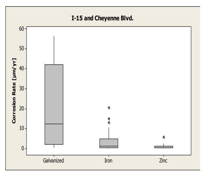
Figure 5-6: Phase II LPR corrosion rate box-plots by element type for I-15 and Cheyenne Blvd.
