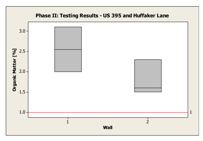
Figure 3-5: Phase II organic content results for US 395 and Huffaker Lane, separated by wall
