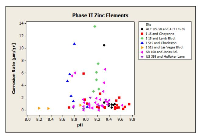
Figure 4-21: Phase II Zinc element LPR corrosion rates as they relate to backfill pH
