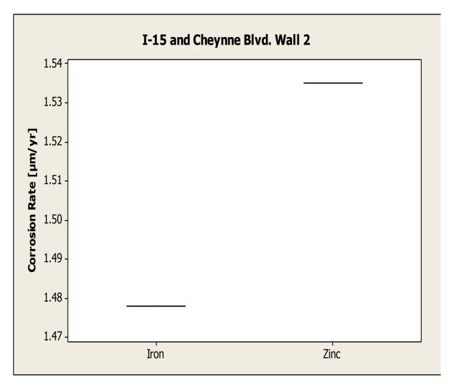
**Figure 5-7**: Phase II LPR corrosion rate box-plots by element type for I-15/ Cheyenne Blvd. Wall 2, figure represent only one data point per type
