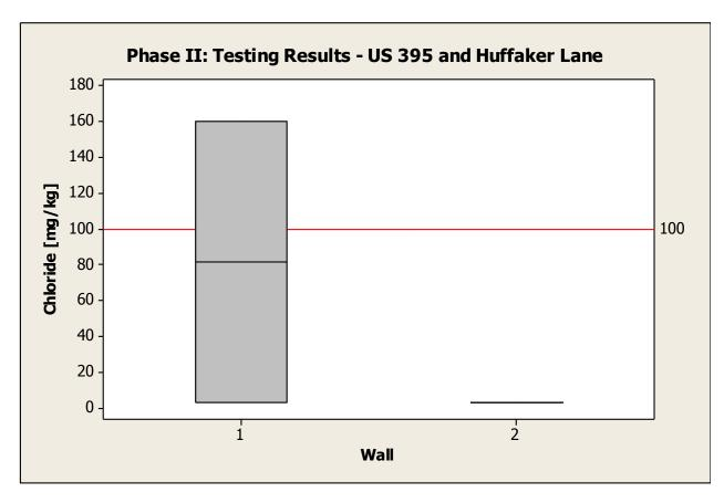
Figure 3-1: Phase II chloride results for US 395 and Huffaker Lane, separated by wall
