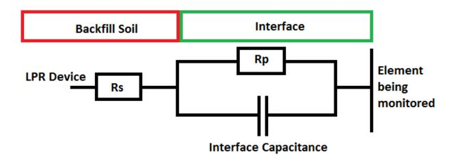
Figure 2-4: Idealized LPR monitoring circuit
