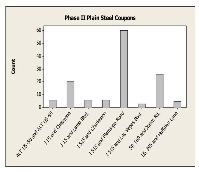
Figure 4-26: Number of plain steel coupons per site for LPR analysis
