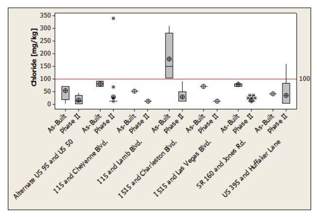
**Figure 3-21**: Comparison of As-built and Phase II soil testing results for chloride content, the majority of all data is below specification.
