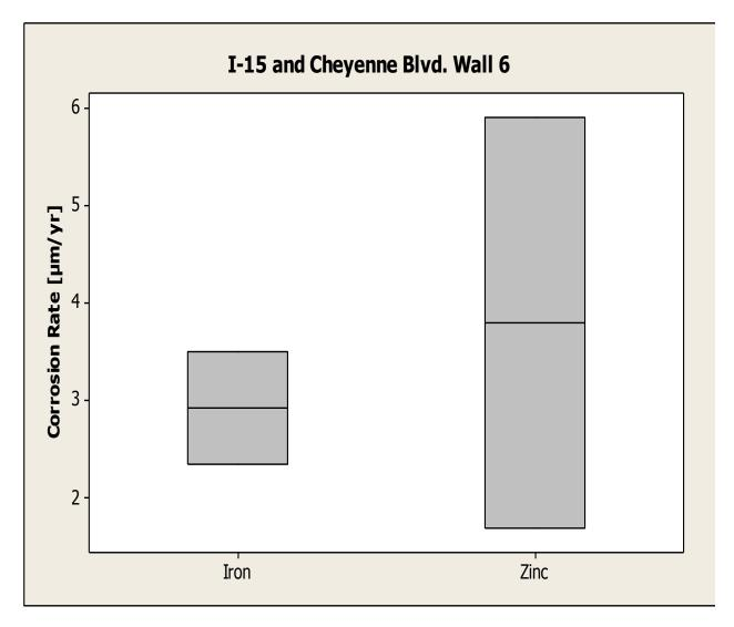
Figure 5-8: Phase II LPR corrosion rate box-plots by element type for I-15/ Cheyenne Blvd. Wall 6
