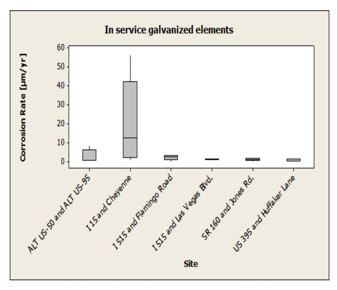
Figure 4-14: Il in-service galvanized corrosion rates distribution information based on site wide information
