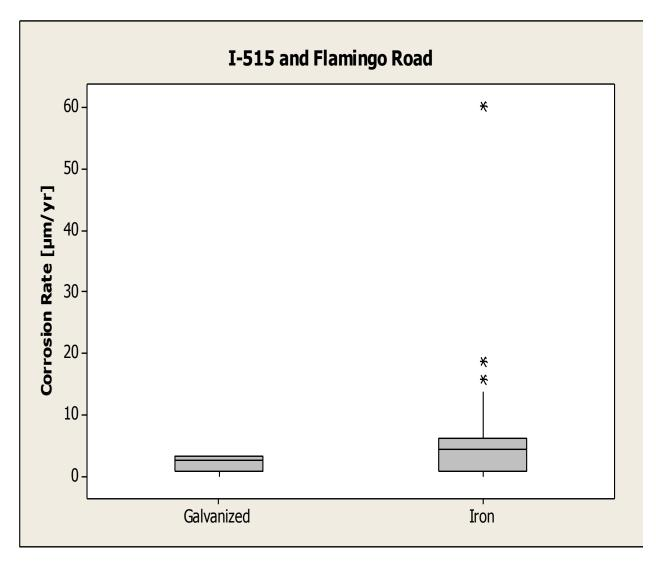
Figure 5-3: Phase II LPR corrosion rate box-plots by element t for I-515/ Flamingo Rd.
