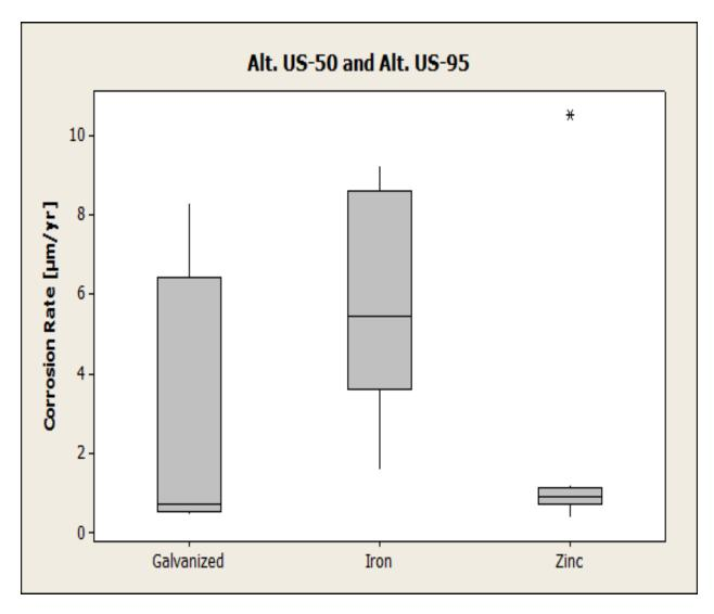
Figure 5-5: Phase II LPR corrosion rate box-plots by element type for Alt. US 50 and Alt. US 95
