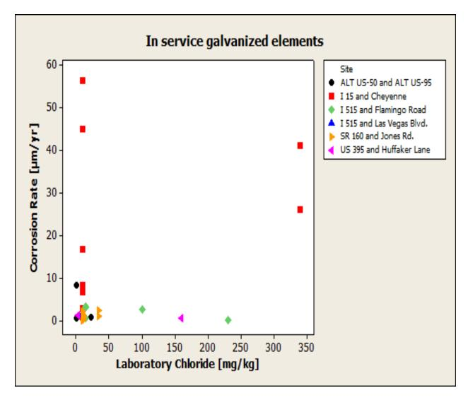
Figure 4-4: Phase II In-service galvanized LPR corrosion rates compared to the chloride content
