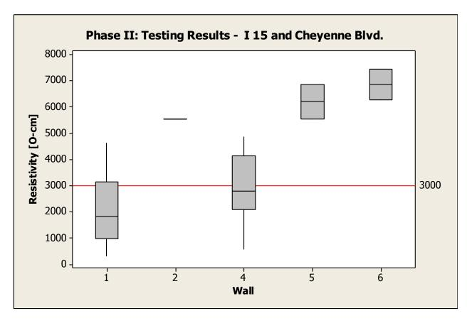
Figure 3-8: Phase II resistivity results for I-15 and Cheyenne Blvd., separated by wall
