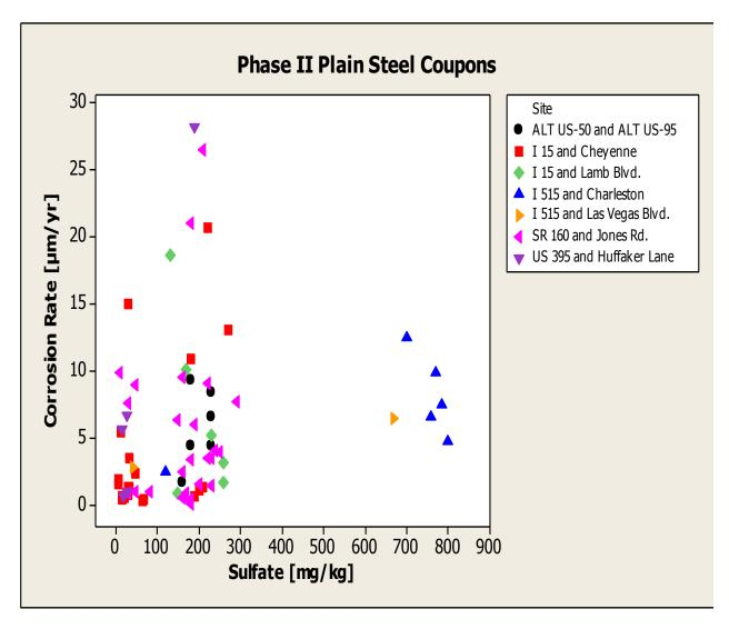
Figure 4-28: Phase II carbon steel coupon LPR corrosion rates with respect to backfill sulfate content.
