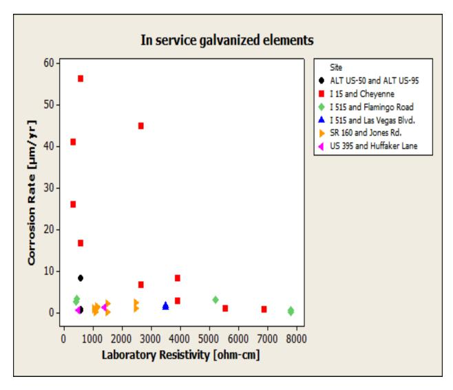
Figure 4-8: LPR corrosion rates compared to the minimum soil resistivity, full spectrum of Phase II
