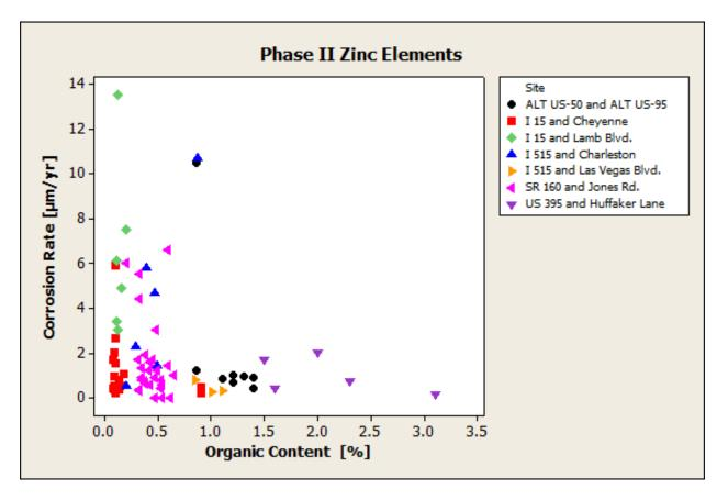
Figure 4-22: Phase II Zinc element LPR corrosion rates as they relate the organic content of the backfill
