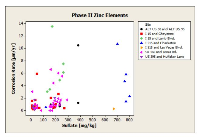
Figure 4-18: Phase II Zinc element LPR corrosion rates compared to the sulfate content
