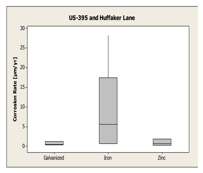
Figure 5-4: Phase II LPR corrosion rate box-plots by element type for US-395 and Huffaker Lane
