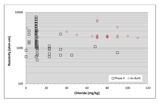
**Figure 3-31**: Relationship between chloride and resistiviy using the combined As-builta and Phase II data, no clear realationship exist.
