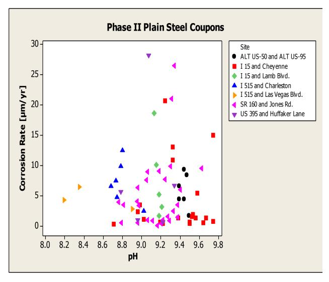
Figure 4-30: Phase II plain steel coupons LPR corrosion rates with respect to backfill pH
