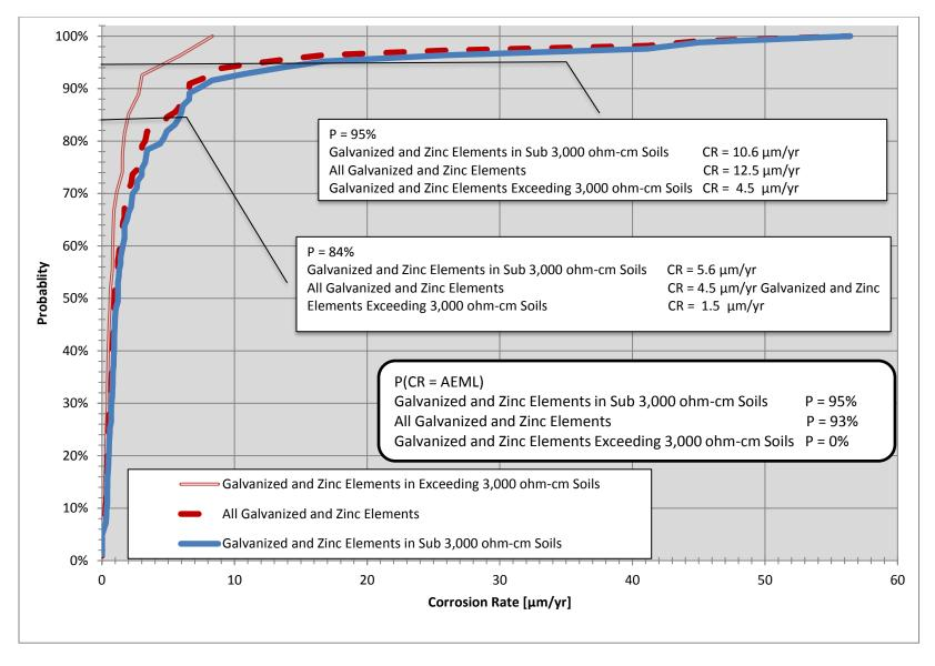
Figure 5-1: Cumulative distribution function (CDF) for the probability that a corrosion rates will exceed a value based on relevant metal types for galvanized in-service soil reinforcements, using all Phase II LPR data
