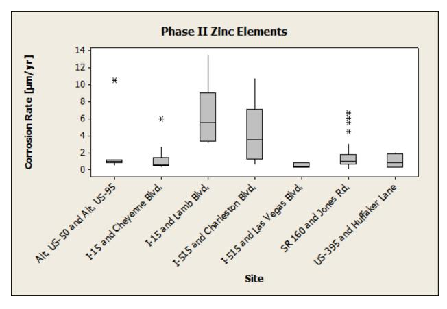
Figure 4-24: Phase II zinc elements corrosion box-plots based on site wide LPR testing results
