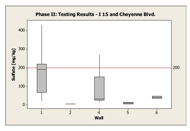
Figure 3-7: Phase II sulfate results for I-15 and Cheyenne Blvd., separated by wall
