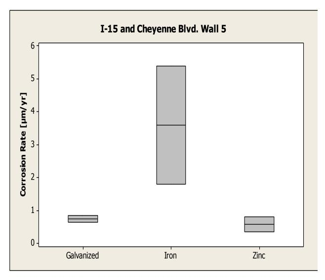
Figure 5-9: Phase II LPR corrosion rate box-plots by element type for I-15/ Cheyenne Blvd. Wall 5
