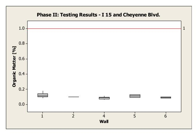
Figure 3-10: Phase II organic content results for I-15 and Cheyenne Blvd., separated by wall
