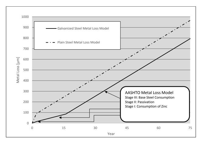
**Figure 4-1**: Nation metal loss models used for the design of sacrificial reinforcement thickness to compensate for metal loss due to corrosion
