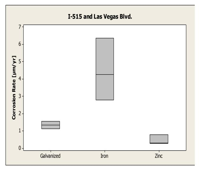
Figure 5-22: Phase II LPR corrosion rate box-plots by element type for I-515/ Las Vegas Blvd.
