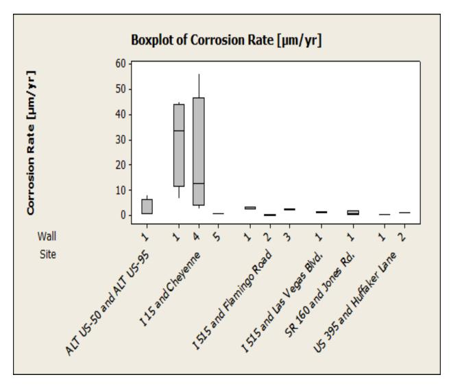
Figure 4-13: Phase II in-service galvanized corrosion rates distribution information based on MSE wall location
