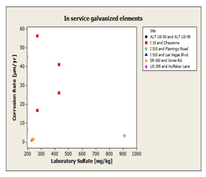
**Figure 4-7**: Phase II LPR corrosion rates and sulfate content data for galvanized in-service elements which FAIL the maximum limit of 200 ppm sulfate
