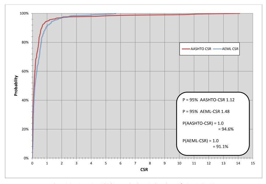
Figure 5-2: Corrosion severity ratio (CSR) CDF curves based on entire Phase II dataset, inflection point CSR ≈ 2.2
