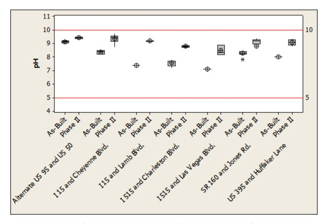
**Figure 3-24**: Comparison of As-built and Phase II soil testing results for pH, all data is within specification, and is narrowly banded as mildly alkaline.
