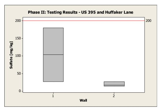
Figure 3-2: Phase II sulfate results for US 395 and Huffaker Lane, separated by wall
