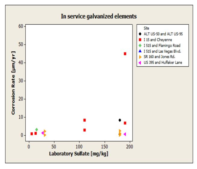
Figure 4-6: Phase II LPR corrosion rates and sulfate content data for galvanized in-service elements which PASS the maximum limit of 200 ppm sulfate
