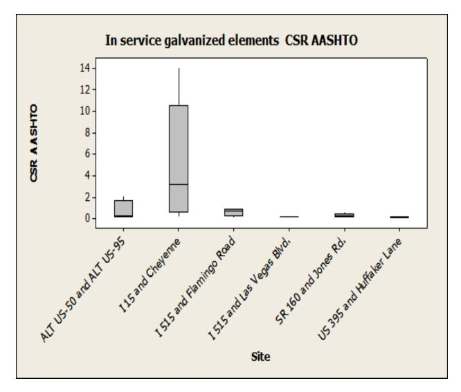
Figure 4-15: In-service galvanized elements CSR values based on site wide information
