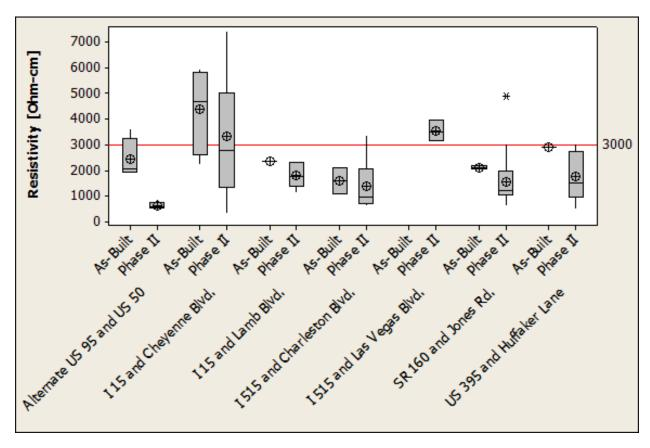
**Figure 3-23**: Comparison of As-built and Phase II soil testing results for minimum soil resistivity. The mean value is indicated with a circle and cross.
