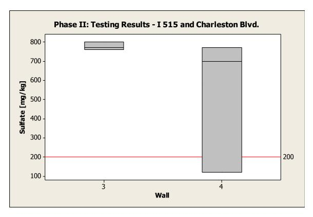
Figure 3-17: Phase II sulfate results for I-515 and Charleston Blvd., separated by wall
