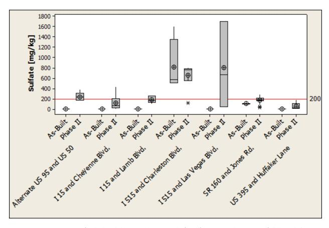
**Figure 3-22**: Comparison of As-built and Phase II soil testing results for sulfate content, the majority of all data is below specification, Charleston Blvd. fails to meet requirements for during either test period.
