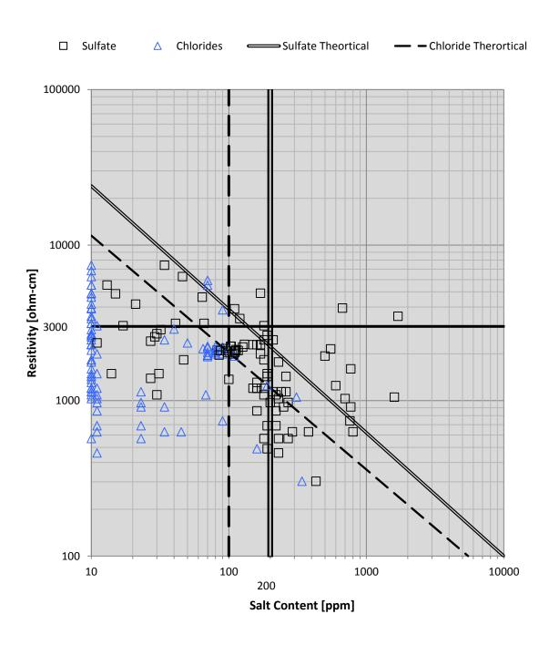
**Figure 3-33**: Phase II salt and resistivity data overlaid on the theoretical resistivity values based on salt content, it is seen that the general trend is for resistivity values measured in Nevada backfills that the resistivity value is below what is predicted using the NACE relationships (solid lines represent specification limits)
