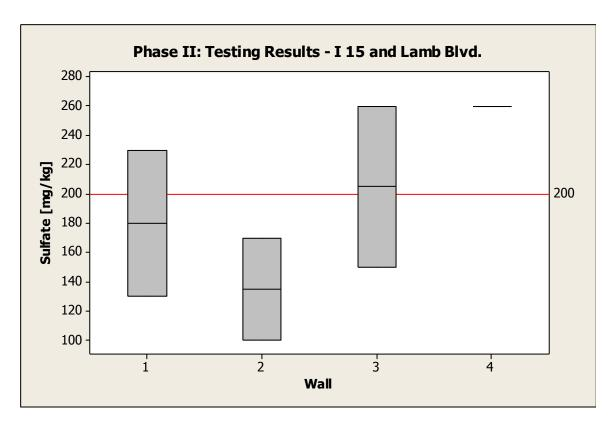
Figure 3-12: Phase II sulfate results for I-15 and Lamb Blvd., separated by wall
