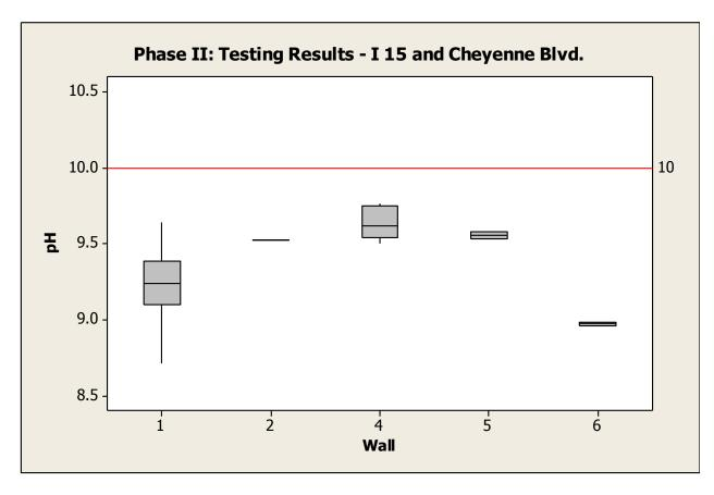
Figure 3-9: Phase II pH results for I-15 and Cheyenne Blvd., separated by wall
