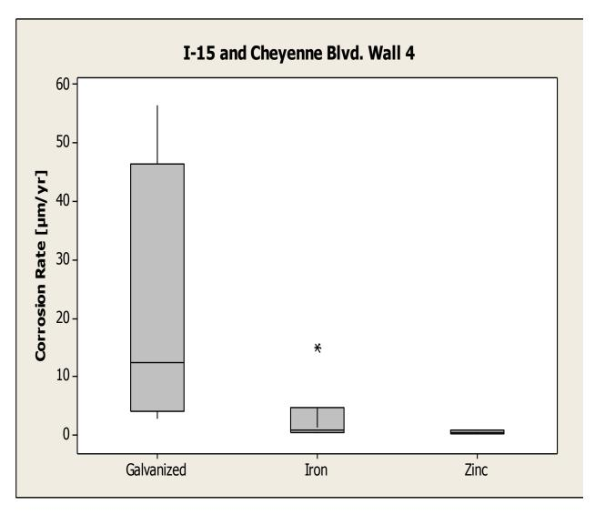
Figure 5-10: Phase II LPR corrosion rate box-plots by element type for I-15/ Cheyenne Blvd. Wall 4
