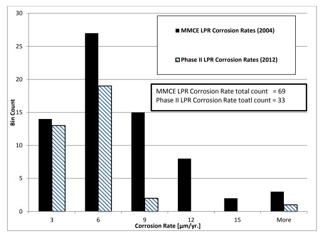
Figure 4-2: Histogram of LPR corrosion rates for both the MMCE and Phase II in-service reinforcements (I-515/Flamingo Rd.)
