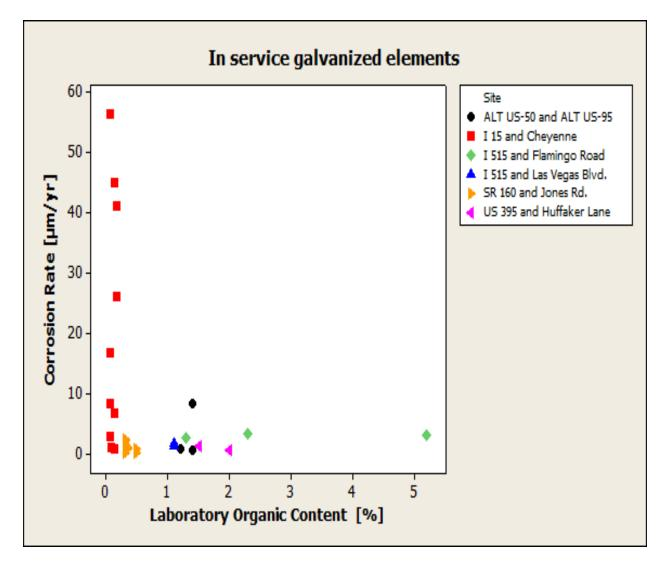
Figure 4-12: II LPR corrosion rates compared with backfill organic content test results
