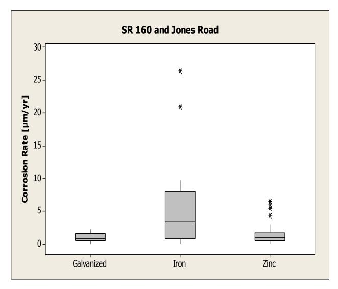
Figure 5-23: Phase II LPR corrosion rate box-plots by element type for SR 160 and Jones
