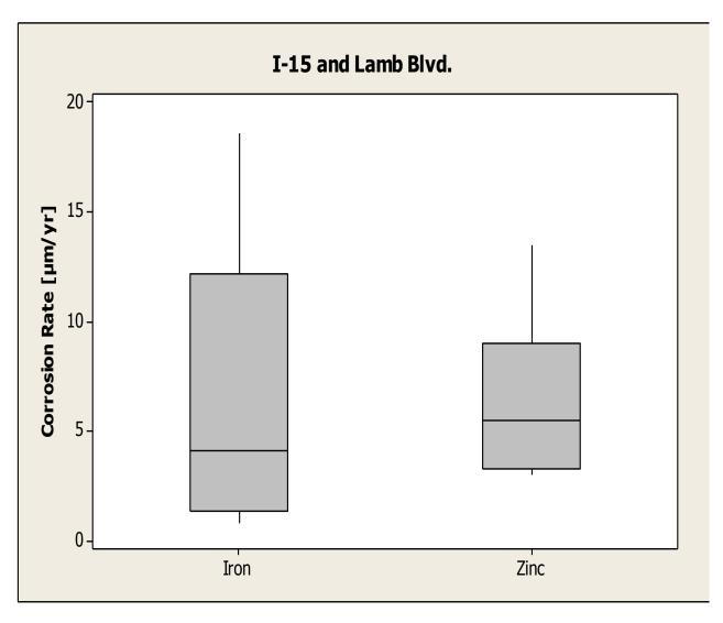
Figure 5-20: Phase II LPR corrosion rate box-plots by element type for I-15/ Lamb Blvd.
