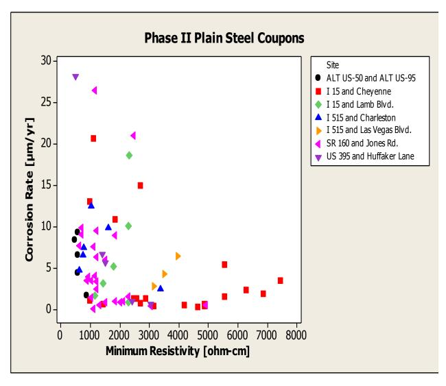
**Figure 4-29:** Phase II plain steel coupons LPR corrosion rates with respect to the minimum soil resistivity, note the pseudorandom trend
