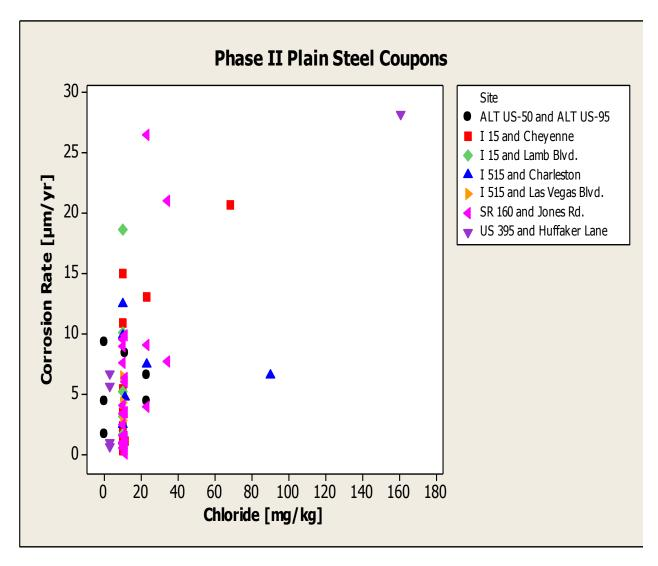
Figure 4-27: Phase II carbon steel coupon LPR corrosion rates with respect to backfill chloride content.
