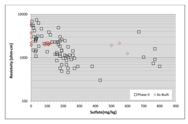
**Figure 3-32**: Relationship between sulfate and resistiviy using the combined As-builta and Phase II data, a weak realationship exist, that mimics the expected inversly porpotional realationsip.
