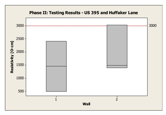
Figure 3-3: Phase II resistivity results for US 395 and Huffaker Lane, separated by wall
