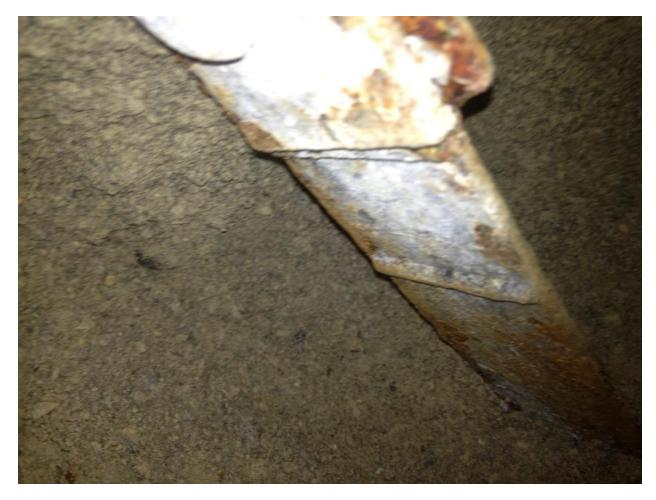
Figure 5-12: In-service galvanized soil reinforcement for I-15/ Cheyenne Blvd. Wall 1, 15 years old.
