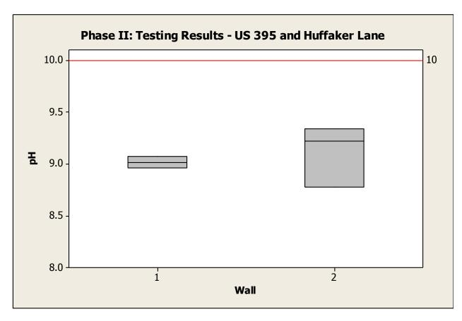
Figure 3-4: Phase II pH results for US 395 and Huffaker Lane, separated by wall
