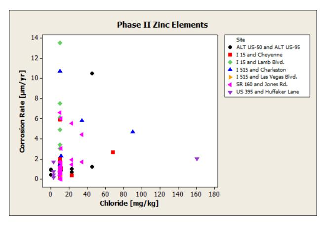
Figure 4-17: Phase II Zinc element LPR corrosion rates compared to the chloride content
