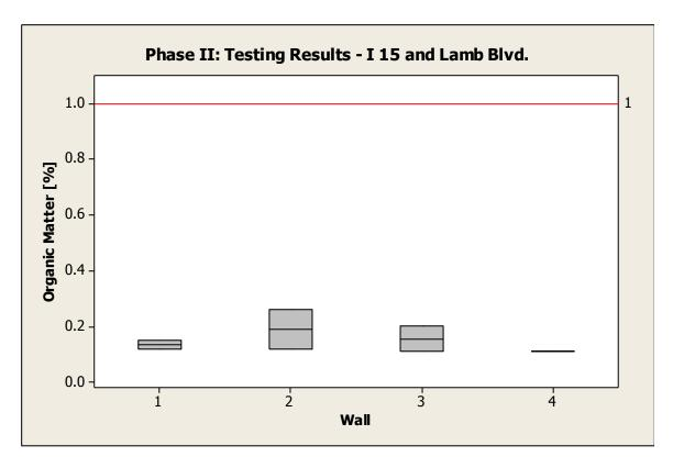
Figure 3-15: Phase II organic content results for I-15 and Lamb Blvd., separated by wall
