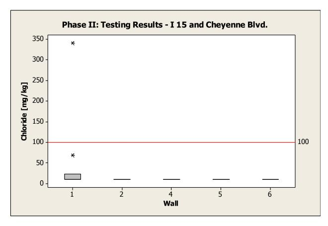
Figure 3-6: Phase II chloride results for I-15 and Cheyenne Blvd., separated by wall
