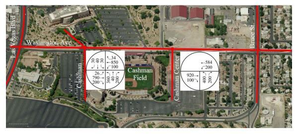
Figure 3.2-5 Simulated Turning Volumes for the New Development Case
