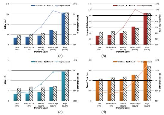
Figure 2.3-14 SCATS Performance for Route Level MOEs – One Direction Detector Failures
