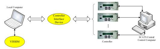
Figure 2.1-1 Hardware-in-the-loop Simulation Environment
