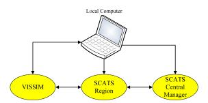
Figure 2.1-2 Software-in-the-loop Simulation Environment
