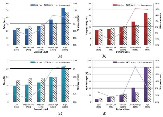
Figure 2.3-16 SCATS Performance for Node Level MOEs - Main Street Detector
