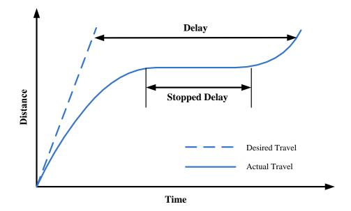
Figure 3.1-2 Illustration of Delay and Stopped Delay
