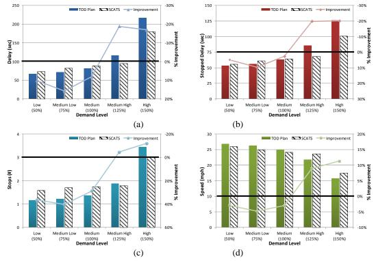
Figure 2.3-15 SCATS Performance for Network Level MOEs - Main Street Detector Failures
