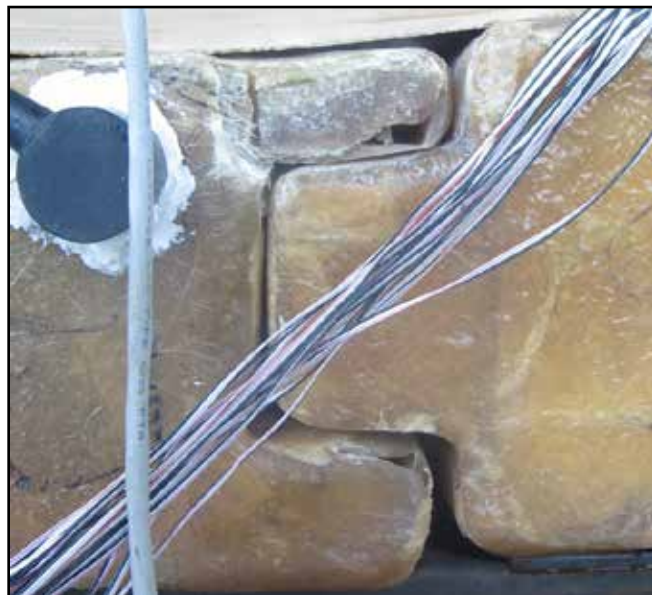
Figure 3.5: Close-Up of Lip-and-Groove Connection Between Two Panels
