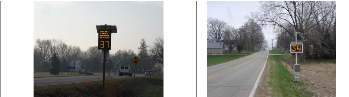
Figure 1: Two different speed signs evaluated for speed reduction in small rural communities in Iowa (image source: CTRE)
