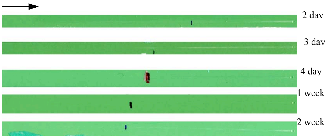
Figure 4.1-8: Scratch test results for coating System 2-3 (DFT = 12mils) after water immersion at 95°C. A normal load range of 1-95N was applied.
