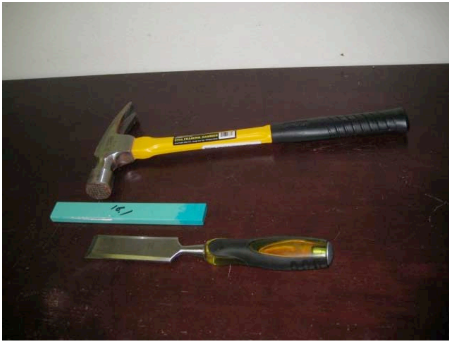
Figure 4.2-2 NCA Test Setup to Generate a Precrack.
