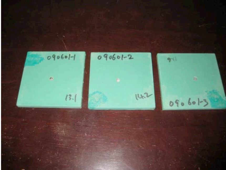
Figure 4.3-1 Wet Disbondment after 12 weeks 95 °C water immersion.
