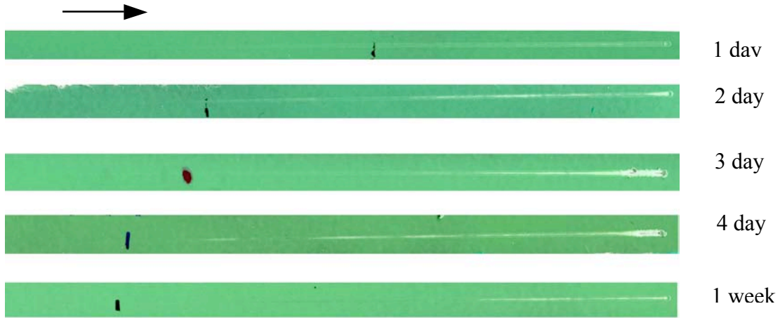
Figure 4.1-6: Scratch test results for coating System 2-1 (DFT = 4mils) after water immersion at 95°C. A normal load range of 1-95N was applied.
