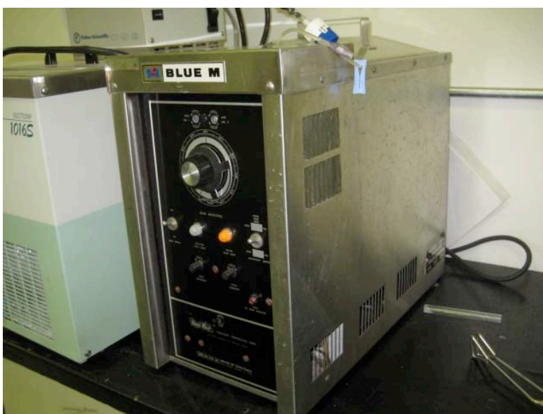
Figure 5.2. Hygrothermal Aging of Coating Samples at 95 °C Water.
