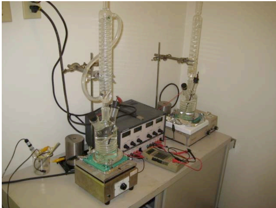
Figure 4.4-1 Cathodic Disbondment Test Setup for 95 °C and 110 °C.
