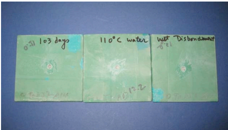
Figure 4.3-2 Wet Disbondment after 103 days 110 °C water immersion.
