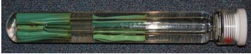
Figure 5.3. Hygrothermal Aging in a Pressure Glass Tube in 110 °C oven.
