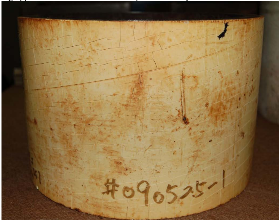
Figure 6-3 Cracking of Thermally Aged 3LPP, at 150 °C for 1,000 hr + 1 wk. In addition to spiral cracking, transverse cracking is also observed.
