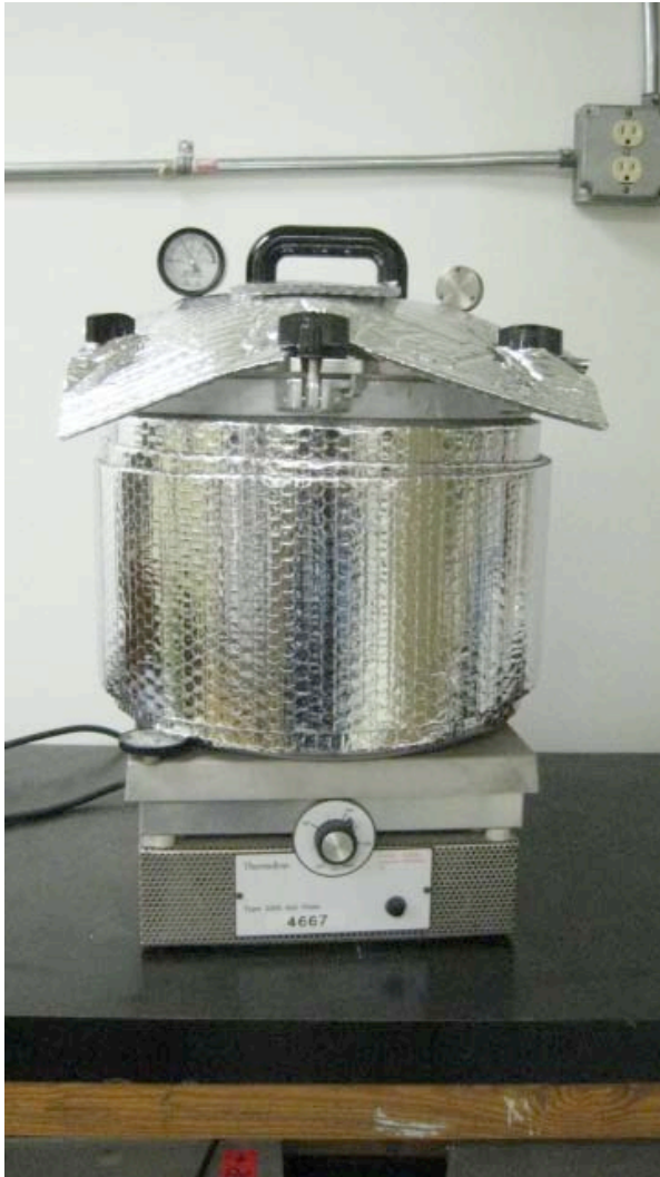
Figure 4-2.6 110 °C Water Immersion of FBE Samples in an Aluminum Autoclave.
