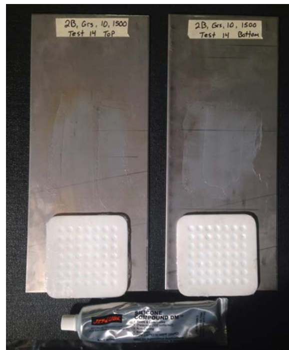
Figure 11.7. Typical grease test; grease was applied to PTFE pads and stainless steel or steel plates
