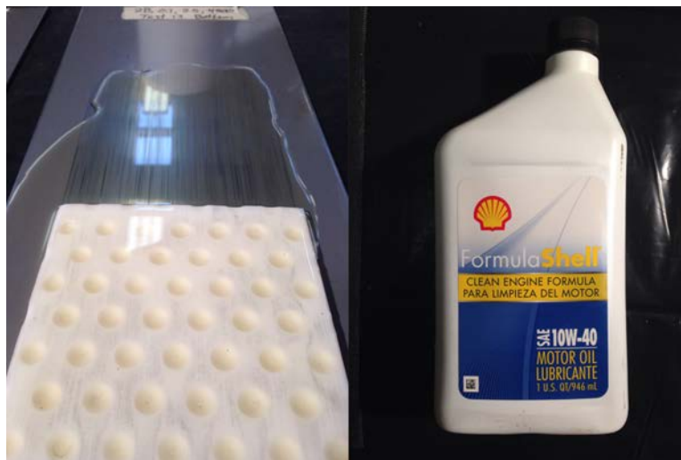
Figure 11.9. Typical oil test; shows oil on PTFE and stainless steel before testing
