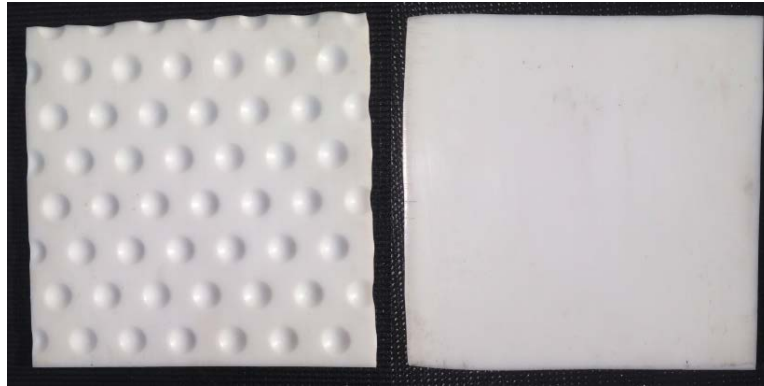
Figure 10.1. PTFE pads; dimpled and smooth
