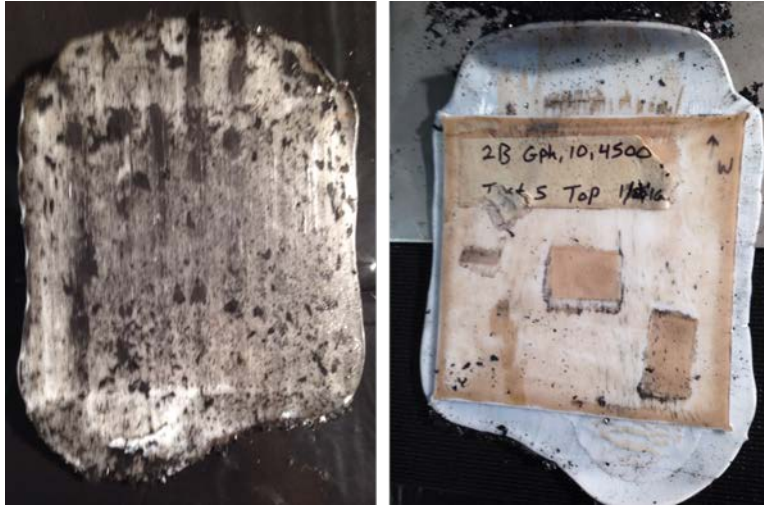
Figure 11.13. Deformed PTFE pad after testing using graphite
