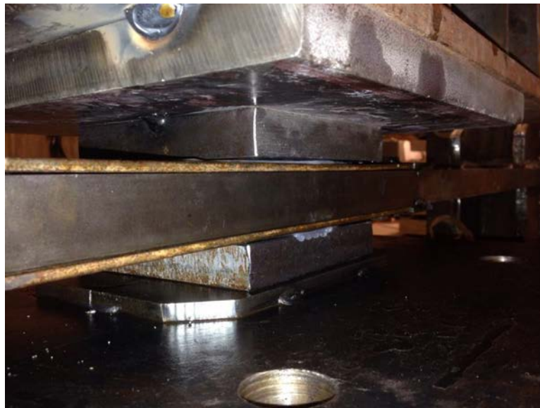
Figure 10.6. Test setup showing PTFE pads attached to steel substrates, and stainless steel sheets attached to steel tongue
