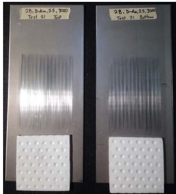
Figure 11.4. Dry test which used dimpled PTFE instead of smooth
