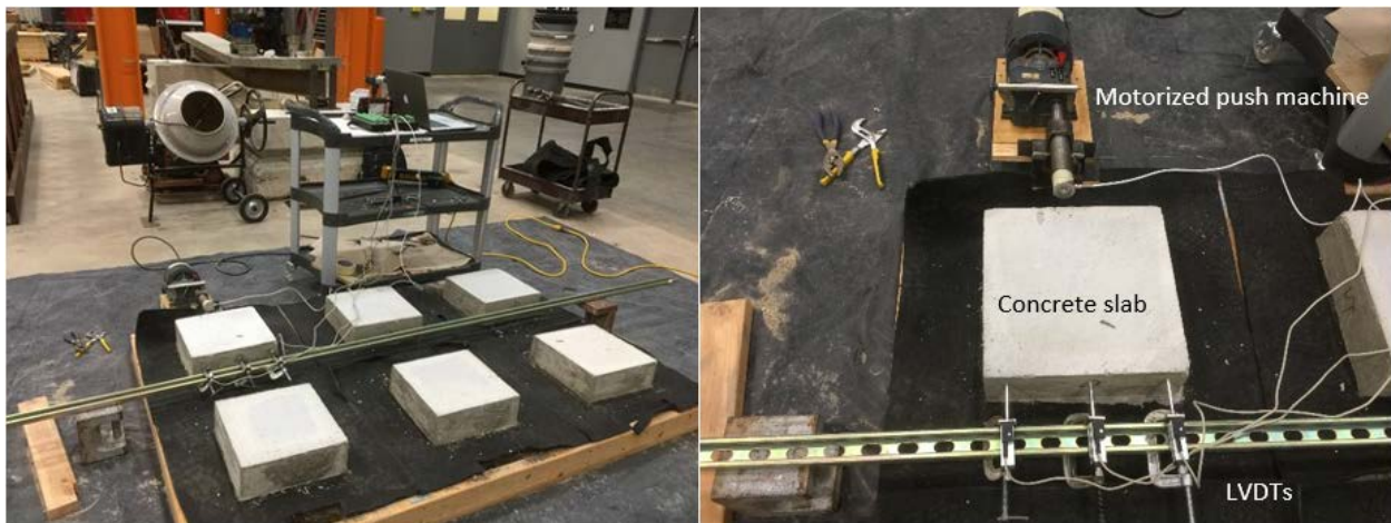
Figure 4.1 Slab/base friction test setup
