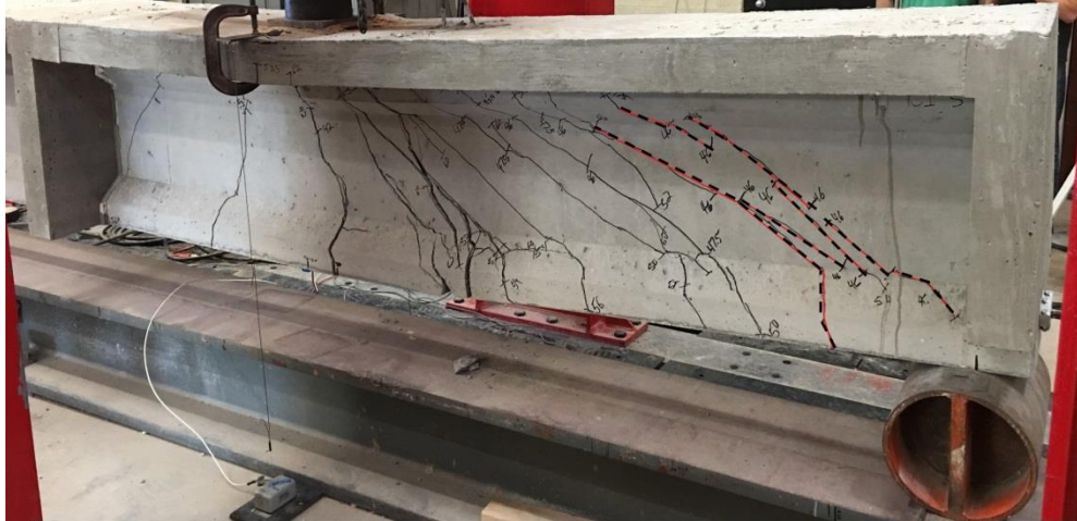
Figure 7.18: Final cracking in test C1s (initial shear cracks highlighted with red and black dashed lines)
