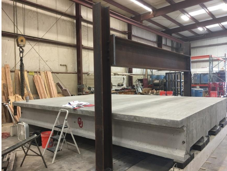
Figure 7.15: Load testing frame over the scaled bridge section
