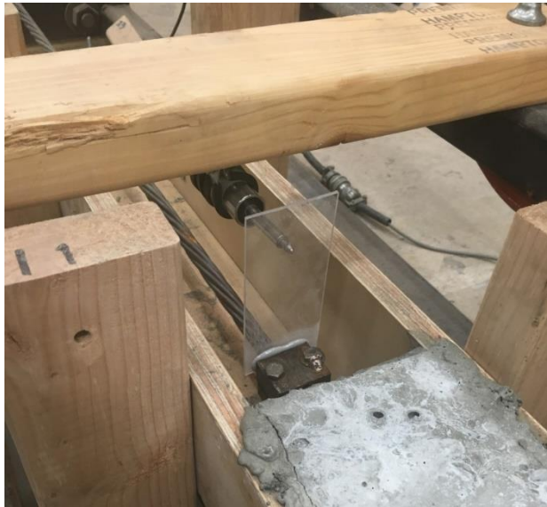
Figure 4.12: LVDT setup on free end of specimen
