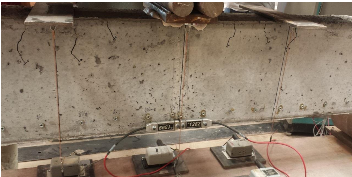
Figure 6.5: Strain gauge placement for SS2-ua
