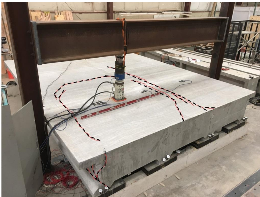
Figure 7.40: Cracking in scaled bridge section slab at failure
