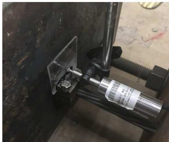
Figure 4.13: LVDT setup on anchored end of specimen
