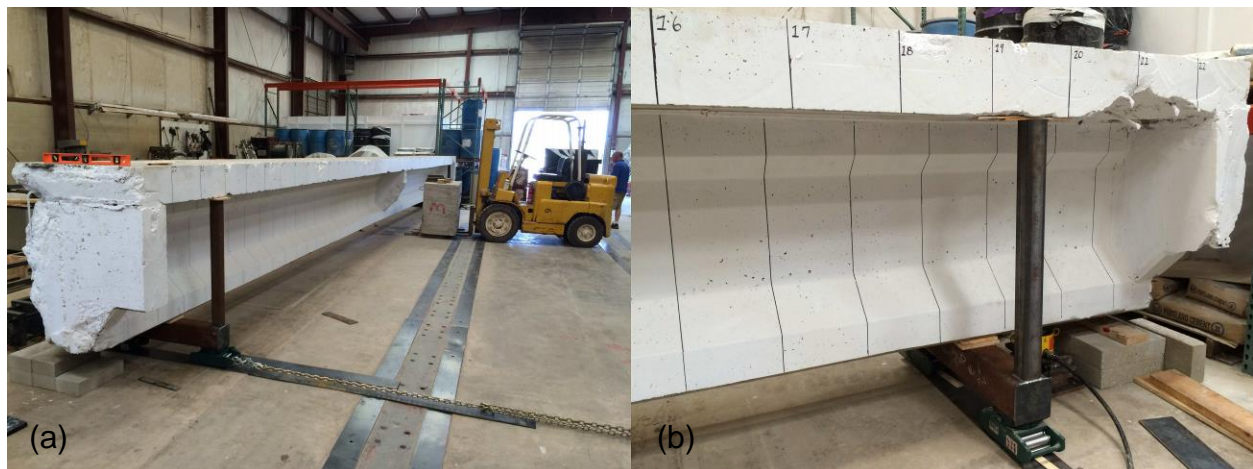
Figure 2.14: (a) Moving of girder C and (b) the gridlines on girder C
