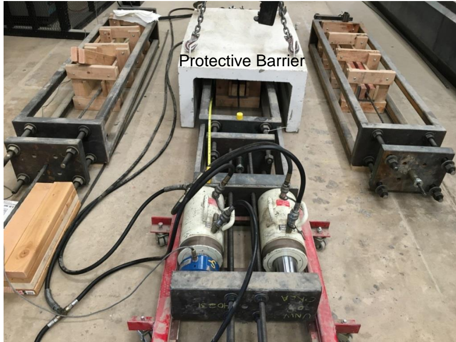
Figure 4.10: Testing setup with protective barrier ready for tensioning
