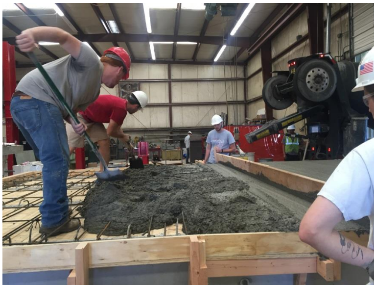
Figure 7.12: Scaled bridge deck construction
