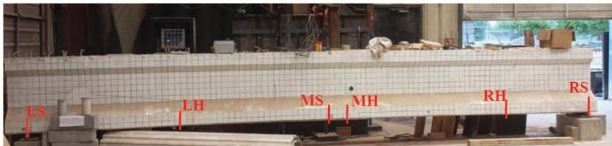
Figure 6.7: Locations for camber measurements
