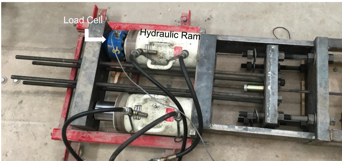
Figure 4.9: Ram assembly with load cell
