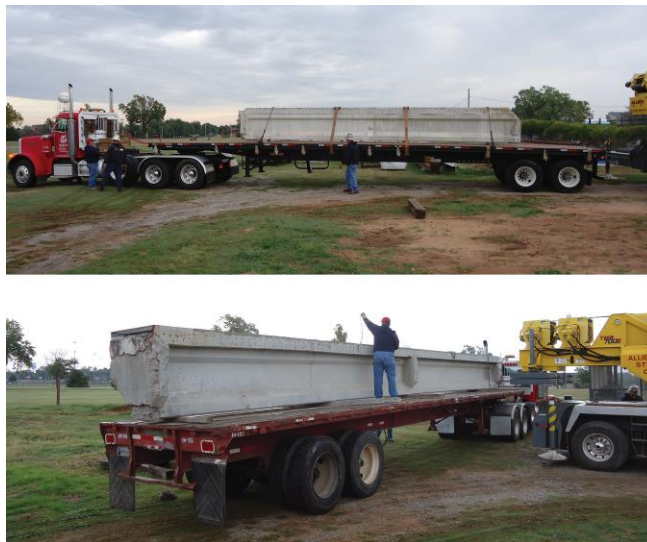
Figure 2.6: Arrival of girders at Fears Lab on flatbed trailers on October 8, 2013
