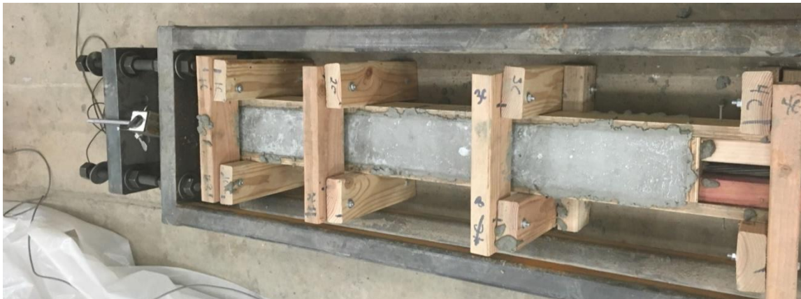
Figure 4.11: Completed casting of bond specimen
