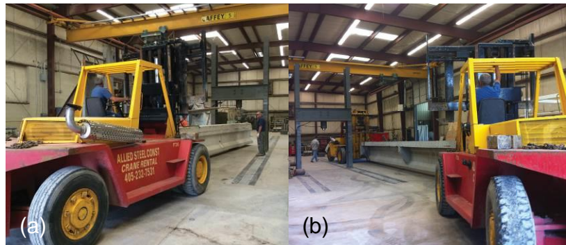
Figure 2.12: (a) Placement of girder A into the load frame at Fears Lab, and (b) girder C into its storage position within the lab
