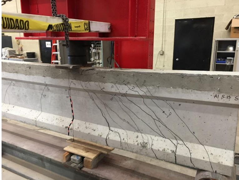
Figure 7.22: Girder A1s cracking patterns, initial cracking shown by red and black dashed line
