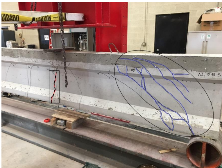
Figure 7.24: Final cracking for specimen A2s, initial flexural crack shown by a red and black dashed line and highlighted by a square, shear cracking at 44.8 kips shown with blue solid lines and highlighted with a circle
