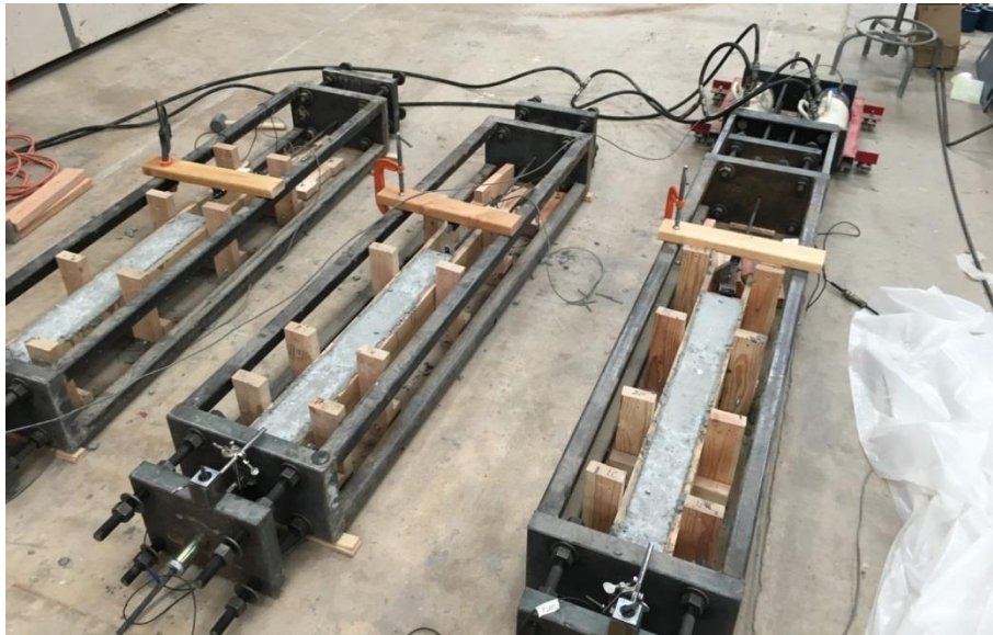
Figure 4.3: Overall bond testing setup
