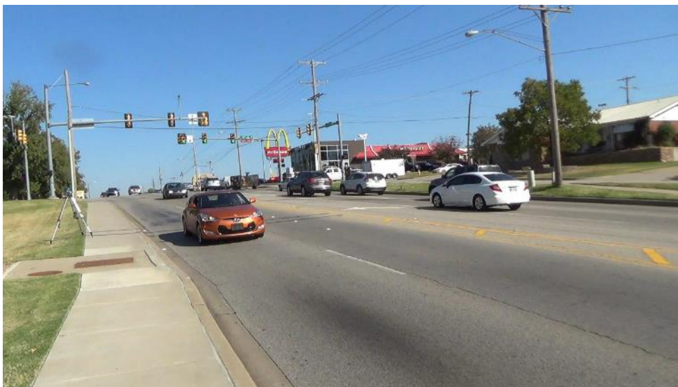
Figure 7-28 Class 2 hybrid car on the edge of lane 2, detected in both lanes
