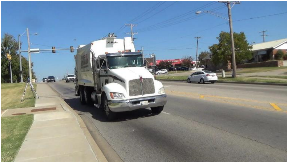
Figure 7-26 Class 6 truck on the edge of lane 2, detected in both lanes
