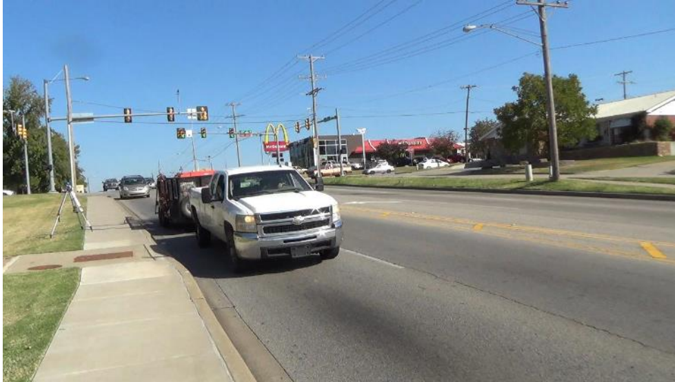
Figure 7-27 Class 3 truck with huge trailer on edge of lane 2, detected in both lanes
