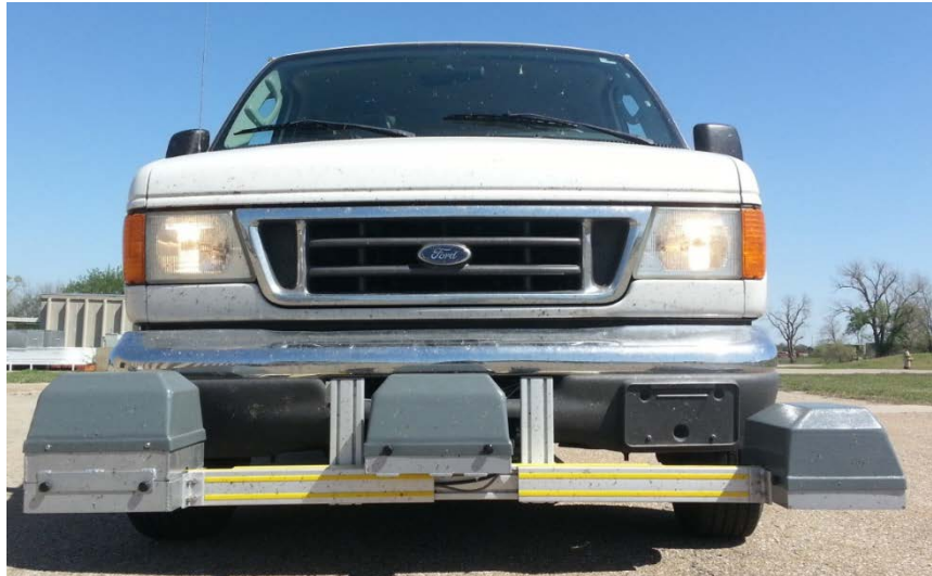
Figure 2.2 AMES 8300 Survey Pro Profiler
