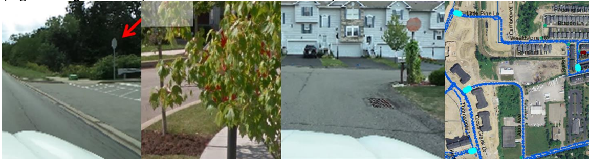
Figure 8 Missed detections. Left: Stop sign facing away from the street. Left middle: Occluded by vegetation. Right middle: Faded. The picture on the right shows stop signs (light blue) that we detected by we were not in the inventory.
