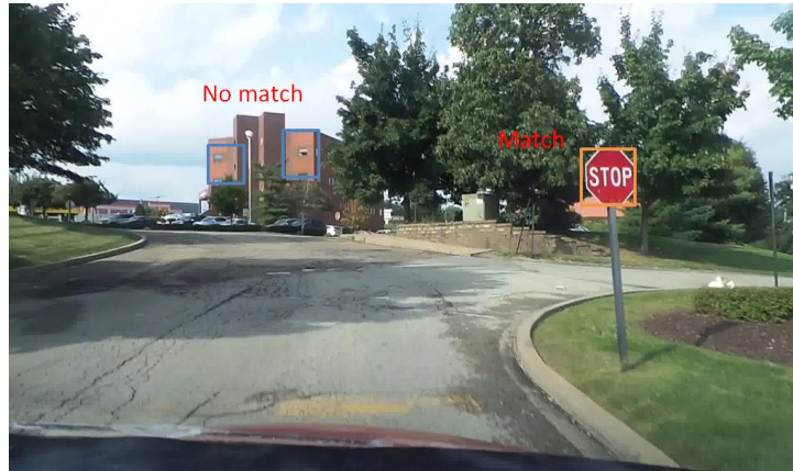
Figure 2 Stop sign detection: First, red areas are detected (boxes). Then the areas are analyzed if they look like a stop sign (orange box) or not (blue boxes).
