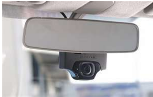
Figure 1. DriveCam Event-Triggered Video Data Recorder
