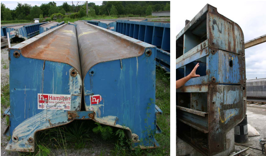
Figure 6.1: NU Girder System Casting Form at Coreslab Structures, Inc.
