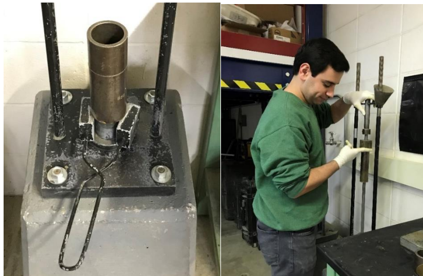
Figure 4. Compaction apparatus for the 2×2 in. specimens
