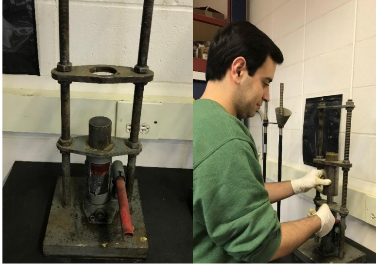
Figure 5. Hydraulic jack for extracting the specimens
