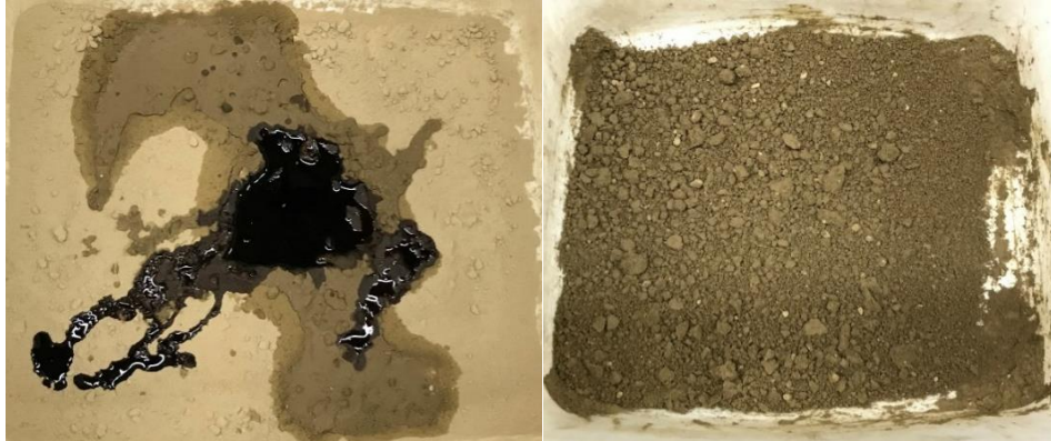
Figure 3. Mixing the loess soil with lignosulfonate
