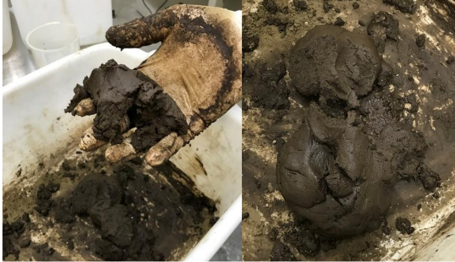
Figure 17. Specimens containing 16% corn oil from Absolute Energy
