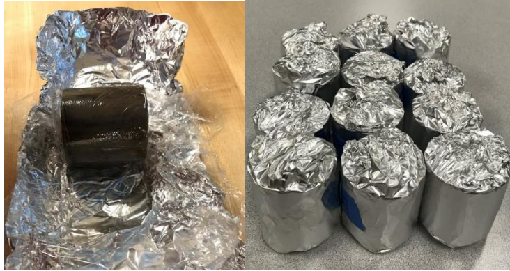
Figure 7. Sealed test specimens in plastic film (left) and aluminum foil (right)
