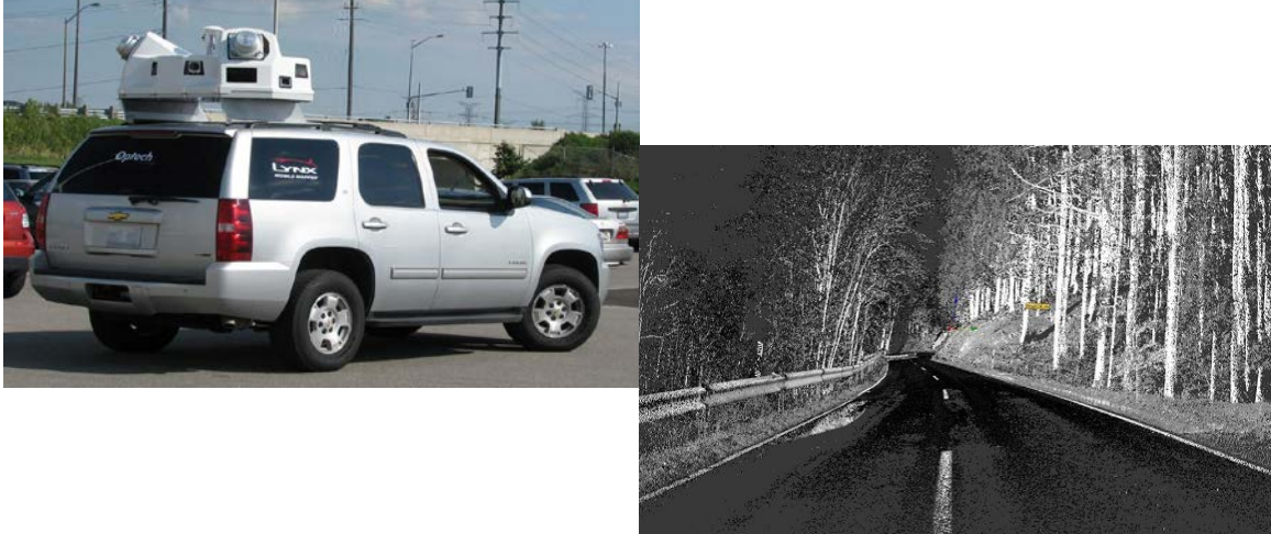
Figure 3 Mobile LiDAR Scanner and 3D points clouds infrastructure
