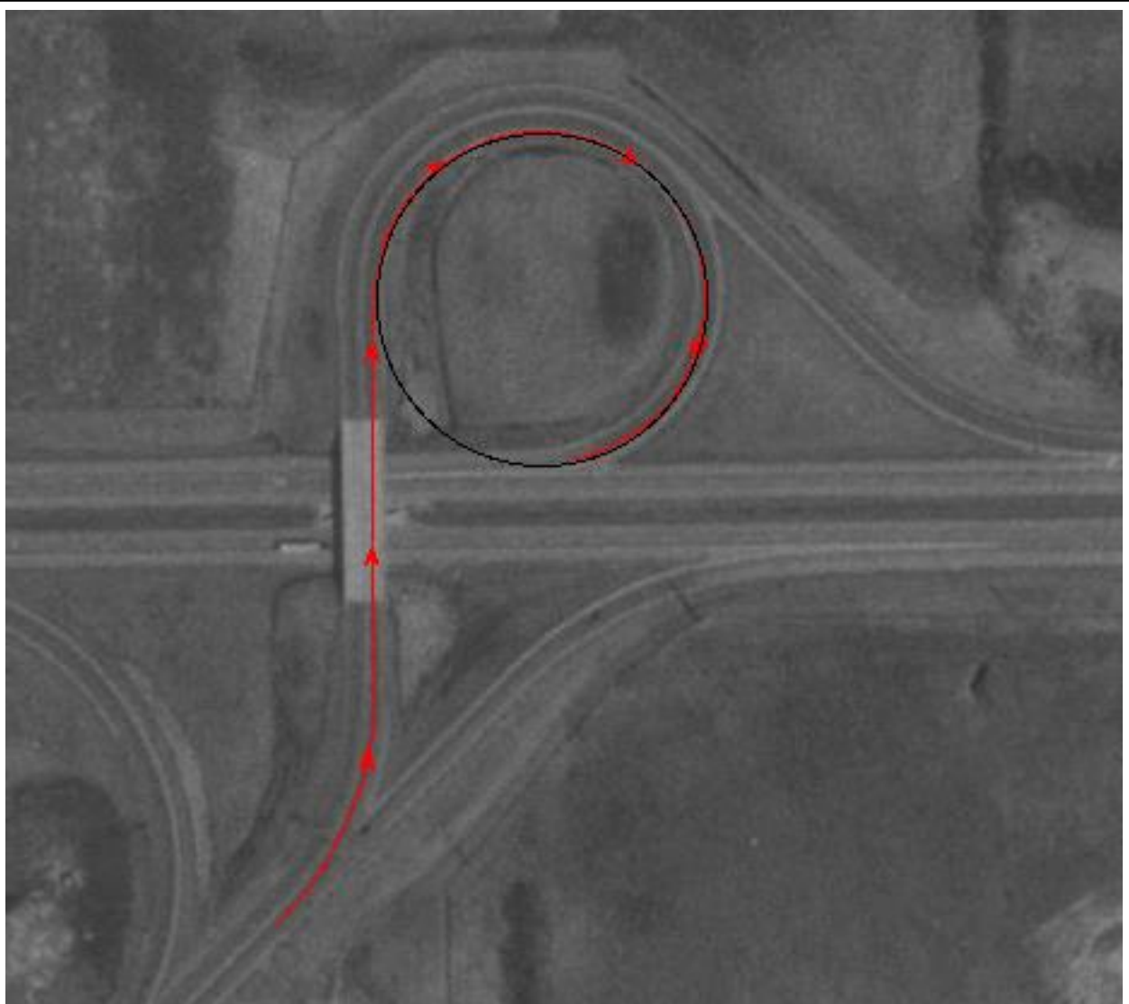
Figure 1. Hot spot 1. The red line indicates the road centerline, as calculated by a spline fit to all passes on this segment. The black circle is an approximation to the spiral part of the onramp.
