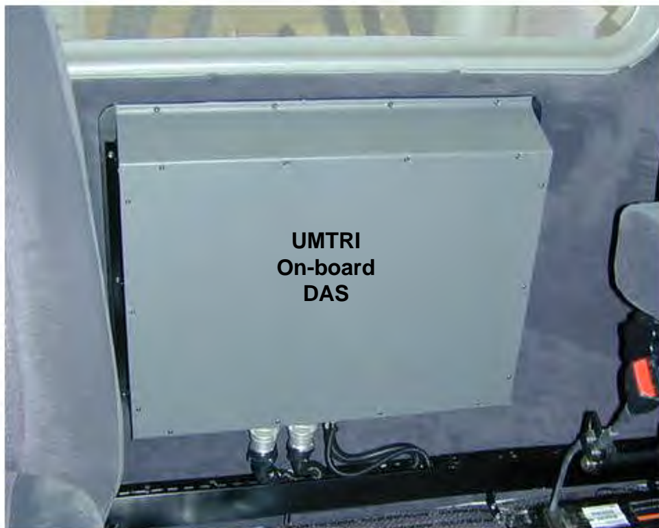
Figure 3-12. Installed UMTRI on-board data acquisition system
