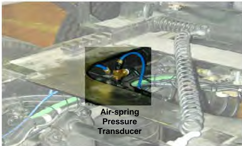
Figure 3-4. Location of air-spring pressure transducer
