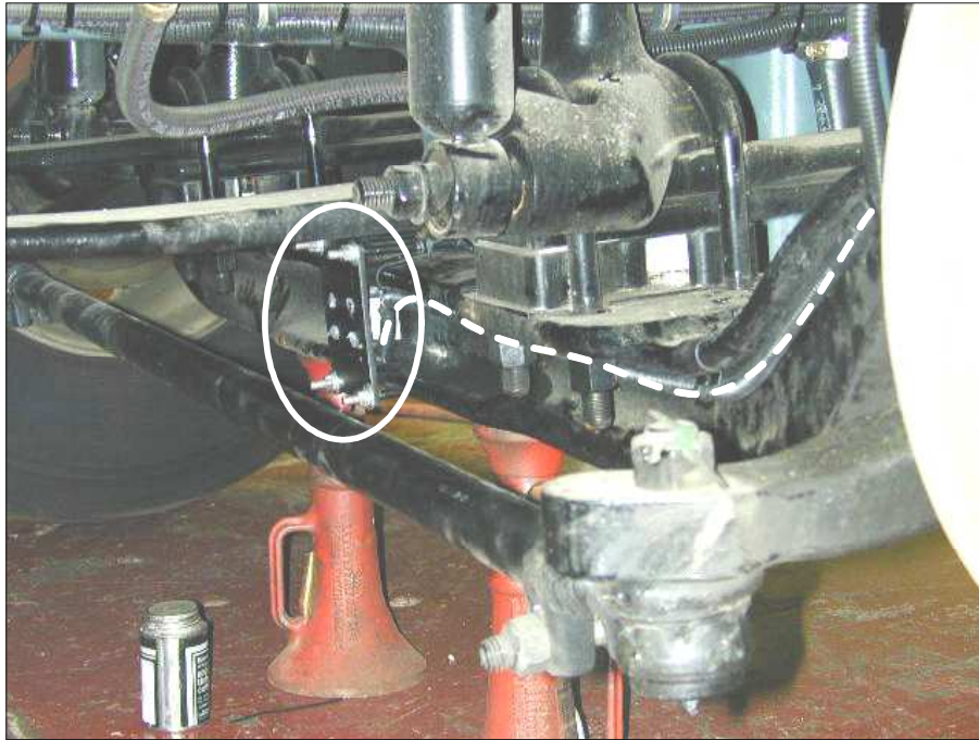
Figure A-E1. Front-axle lateral accelerometer housing, mount, wiring path and location.
