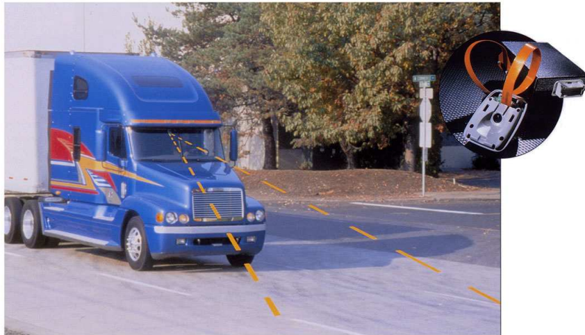
Figure 4-1: The Lane Guidance™ windshield mounted camera and additional CPU (both shown in corner) process forward viewing images of the lane markings to detect if the vehicle is drifting out of the lane of travel
