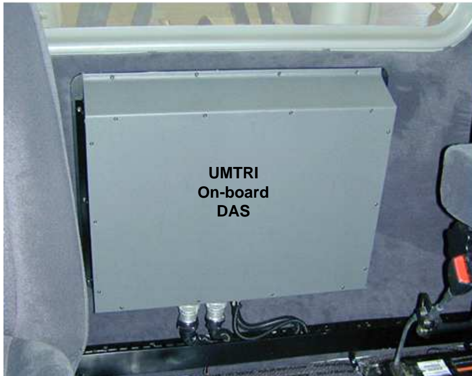
Figure 3-12.: Installed UMTRI on-board data acquisition system
