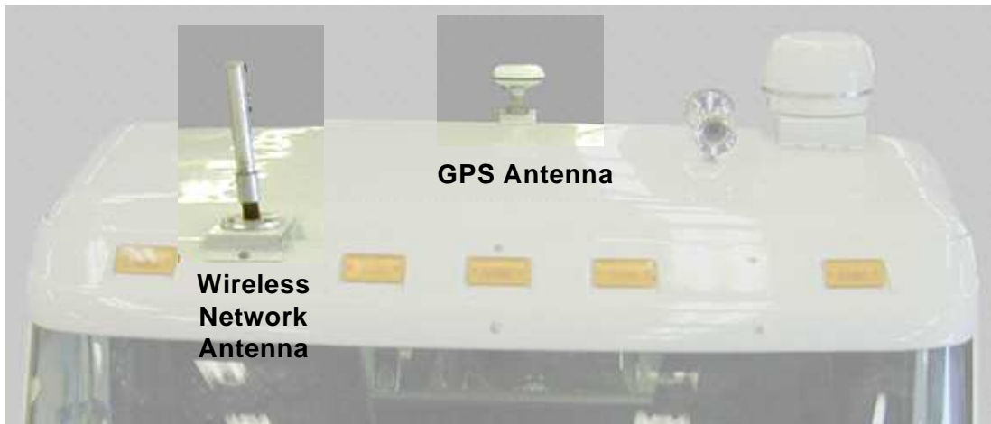
Figure 3-7: Location of wireless network and GPS antennas
