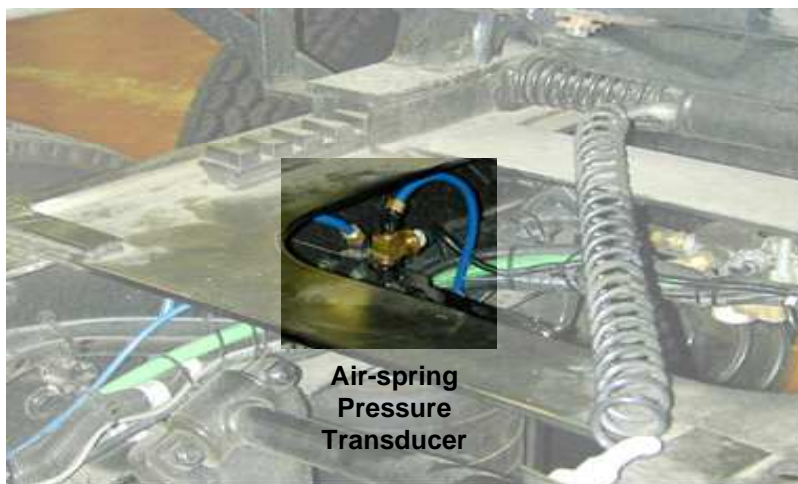
Figure 3-4: Location of air-spring pressure transducer
