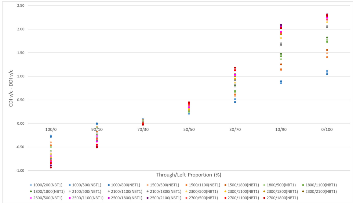
Figure E - 9: Difference in v/c ratios between CDI and DDI on NBT1 at different traffic demands and through/left proportions for LC2
