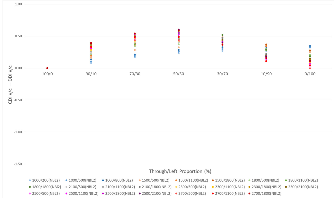
Figure E - 22: Difference in v/c ratios between CDI and DDI on NBL2 at different traffic demands and through/left proportions for LC3
