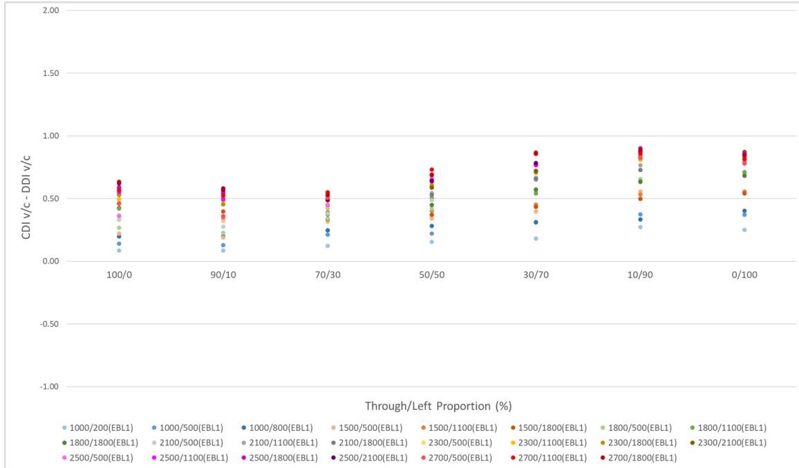
Figure E - 4: Difference in v/c ratios between CDI and DDI on EBL1 at different traffic demands and through/left proportions for LC1
