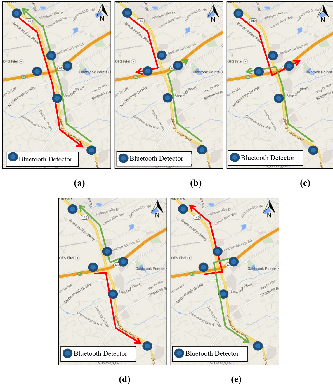
Figure A - 3: The 10 Travel-time routes used for multiple distribution analysis, (a) northbound (NB) and southbound (SB) routes through the interchange, (b) NB and SB right turn onto I-85, (c) NB and SB left turn onto I-85, (d) right turns originating from I-85, and (e) left turns originating from the interchange
