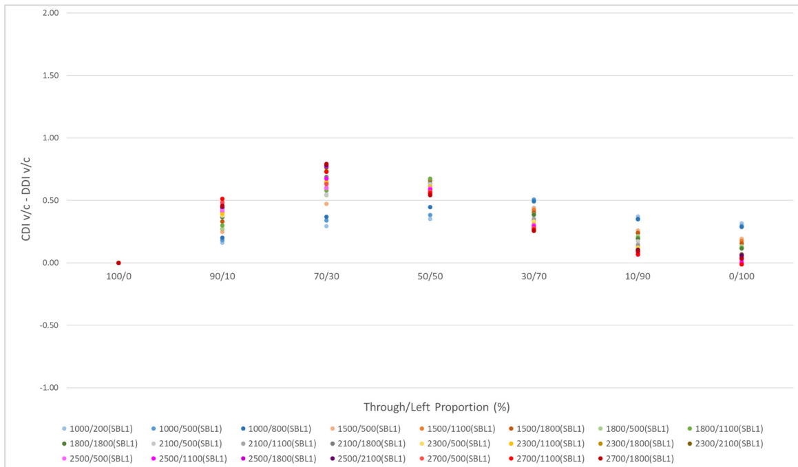
Figure E - 3: Difference in v/c ratios between CDI and DDI on SBL1 at different traffic demands and through/left proportions for LC1
