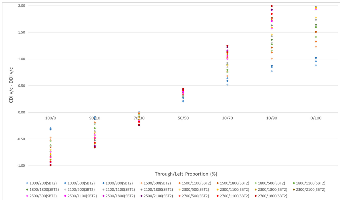
Figure E - 7: Difference in v/c ratios between CDI and DDI on SBT2 at different traffic demands and through/left proportions for LC1
