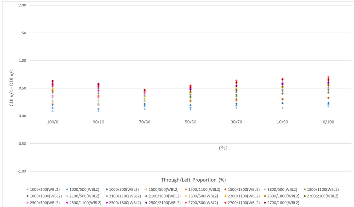
Figure E - 8: Difference in v/c ratios between CDI and DDI on WBL2 at different traffic demands and through/left proportions for LC1
