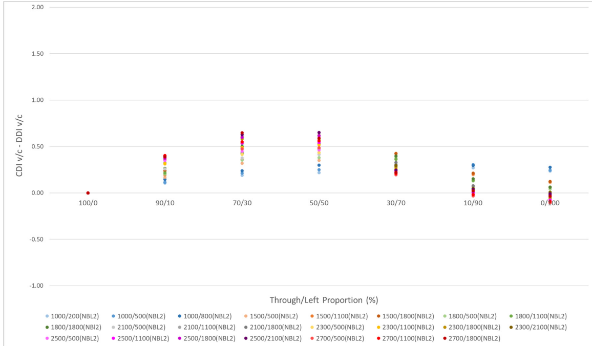
Figure E - 6: Difference in v/c ratios between CDI and DDI on NBL2 at different traffic demands and through/left proportions for LC1
