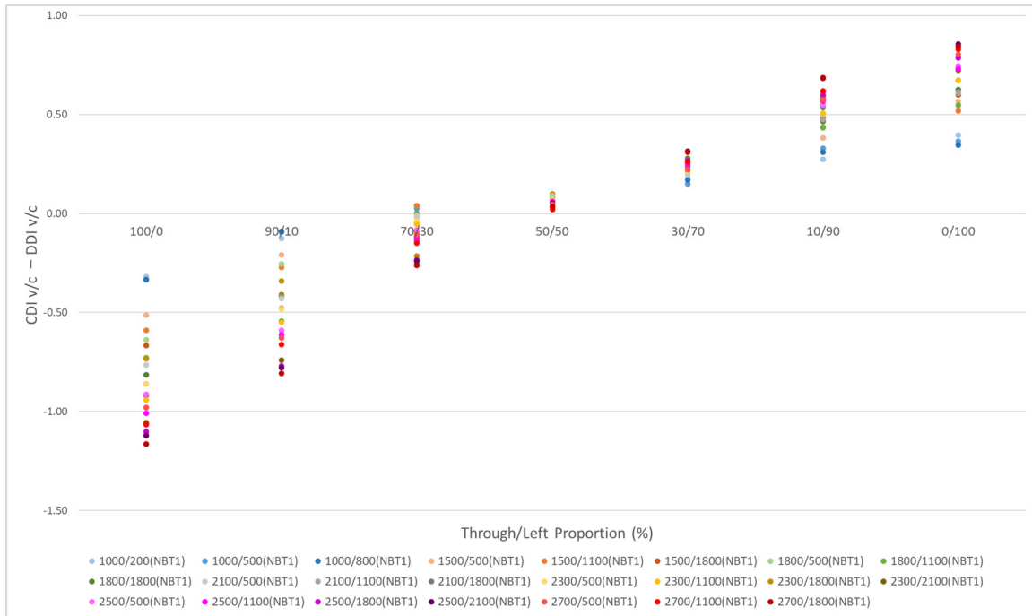
Figure E - 17: Difference in v/c ratios between CDI and DDI on NBT1 at different traffic demands and through/left proportions for LC3
