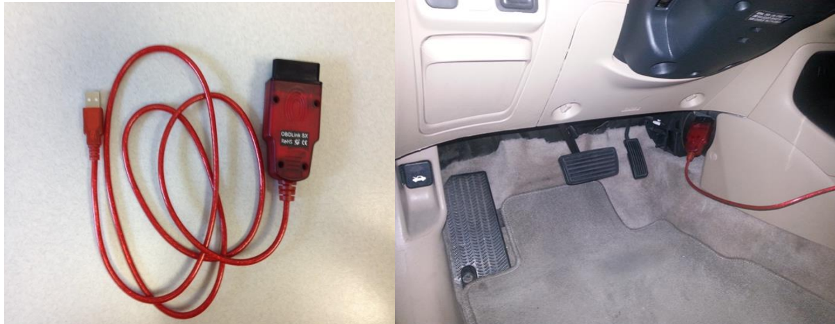
Figure 3-3. (a) OBDLink SX ® Scan Tool cable and (b) cable attached to the OBD-II port of test vehicle
