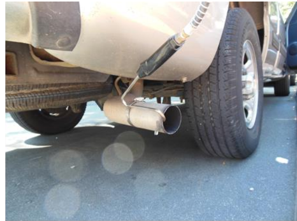
(b) PEMS Exhaust Sampling Line Connected to the Vehicle Exhaust Pipe
