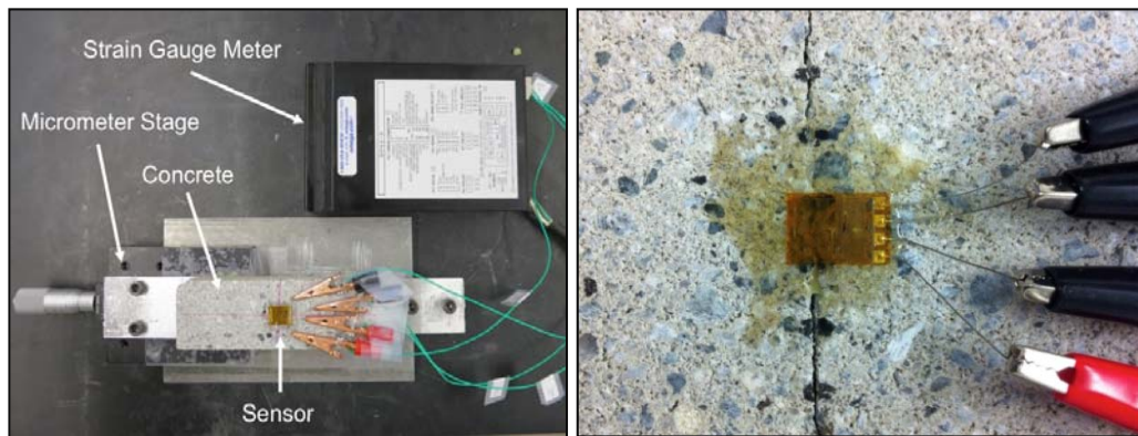
Figure 10. Left: top view of the experiment setup. Right: positioning of the sensor 90° to the crack (source: Tung et al. 2014, see journal papers in Conclusions).
