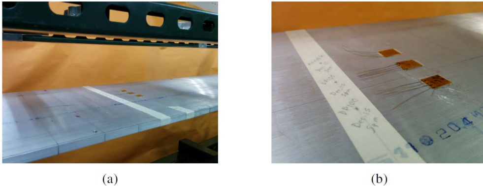
Figure 15. Strain transfer test: (a) global view to beam with sensors, and (b) detail of sensors.
