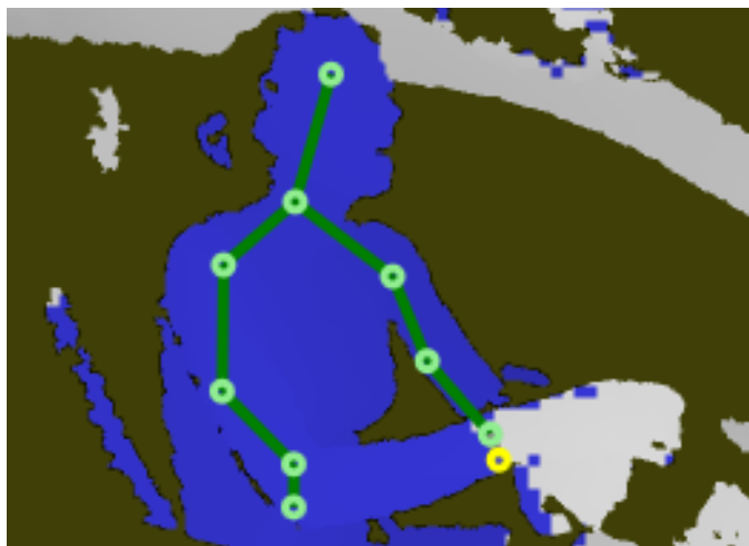
Figure 3: Example of the skeleton model that was erroneously fit to an arbitrary frame of the depth sequence by the skeleton tracker provided with the Microsoft Kinect SDK.
