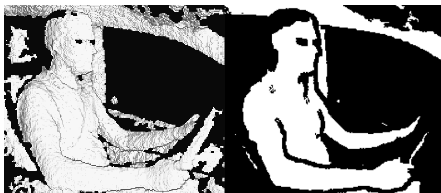
Figure 2: Left: Visualization of a depth frame. Right: The corresponding mask with enhanced boundaries between objects, computed using our framework.
