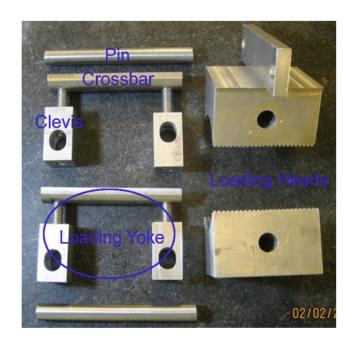
(a) Loading assembly Figure D-1. Original loading device.
