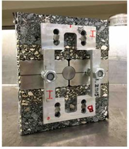
(b) Assembled CSIC specimen Figure D-5. New specimen assembly.
