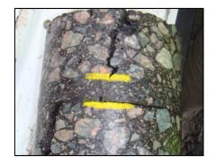
Figure 5-6. Crack jumping phenomenon (Bennert et al., 2011)
