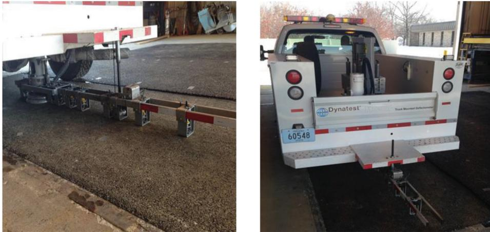
**Figure 3.28** Falling weight deflectometer and test set-up.
