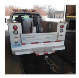
Figure 3.28 Falling weight deflectometer and test set-up.
