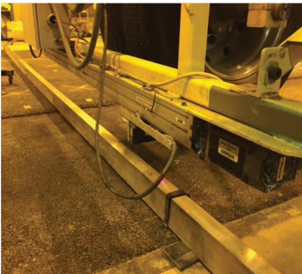
Figure 3.19 Automated laser profile system.
