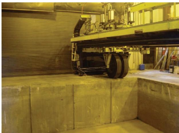
**Figure 3.1** APT loading machine and empty test pit (Levenberg et al., 2009).
