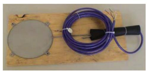
Figure 3.13 Geokon model 3500 earth pressure cell.
