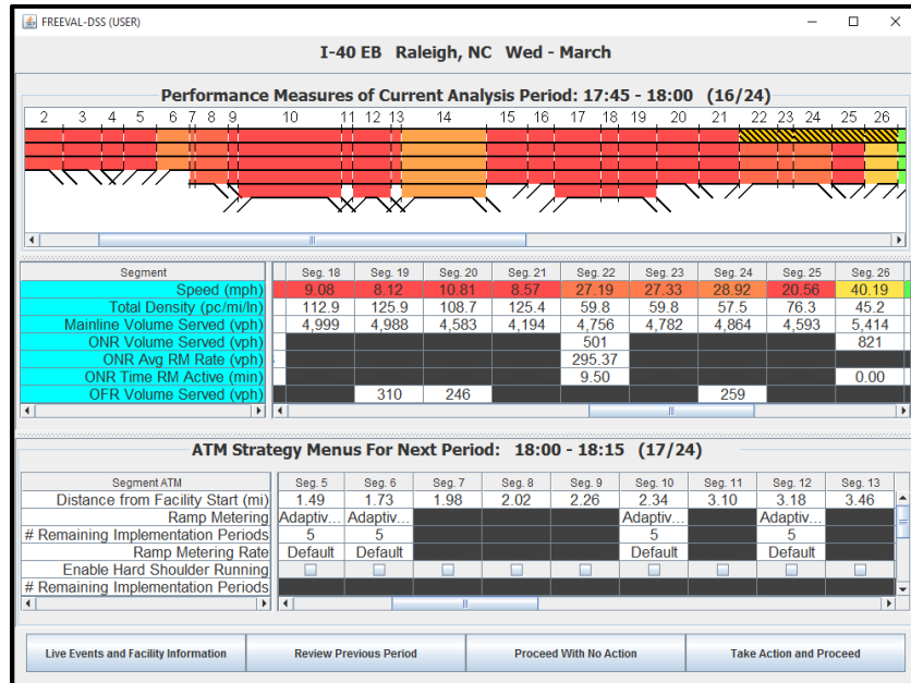
Figure 5-20. Poor facility conditions still exist when the first ramp metering intervention is set to expire so the strategy is extended for an additional 5 analysis periods.
