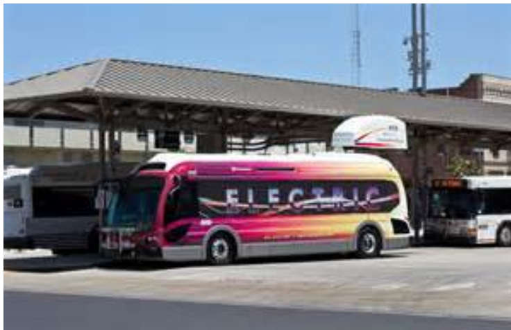
Figure 1. Proterra bus overhead charging station
