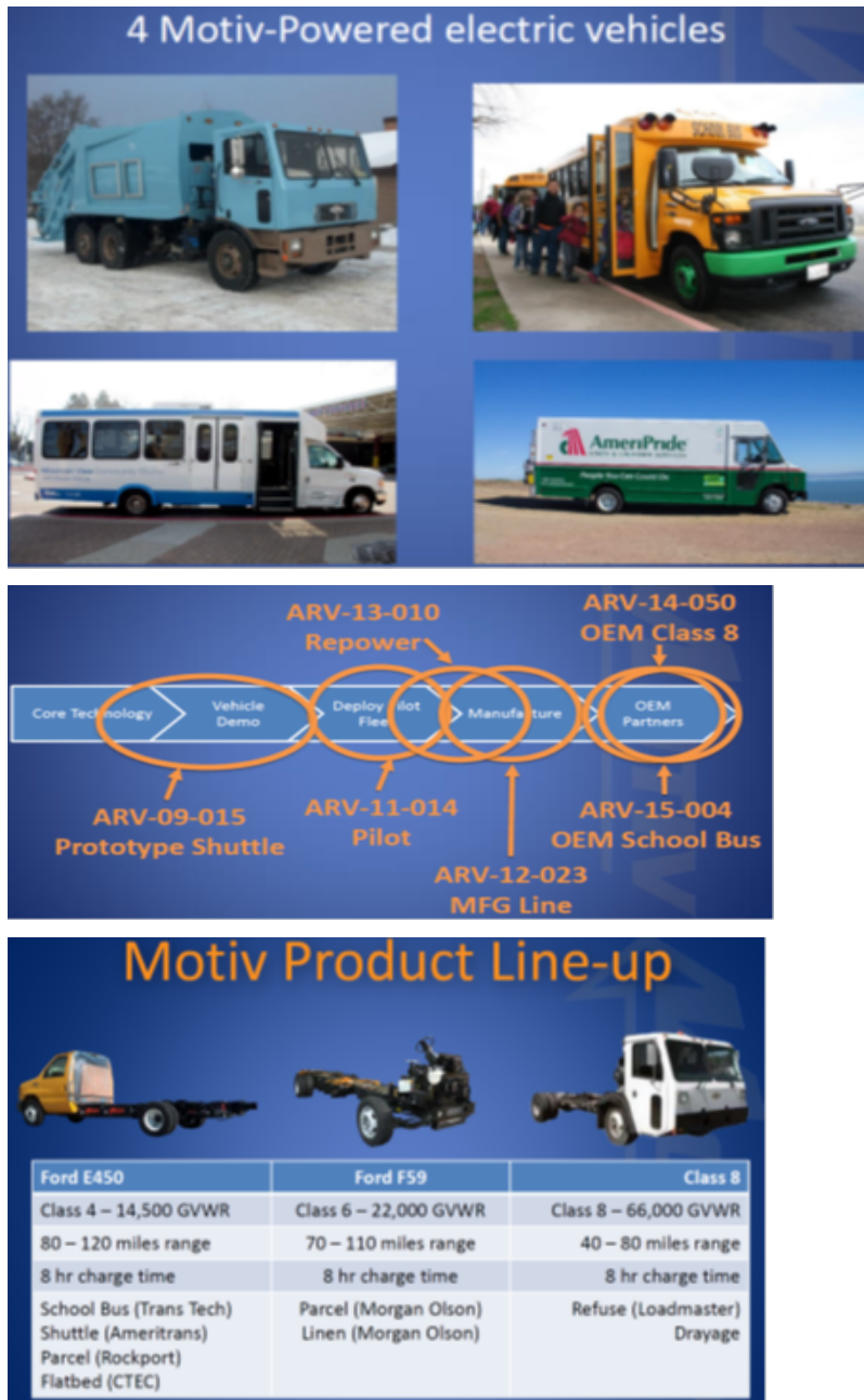
Figure 21. Motiv Power: Example of vehicles in demonstration phase (top), including a refuse truck, a school bus, an “Eco-Charge” community shuttle, and a delivery truck; From pilot to commercial diagram (center); and Three primary chassis underlying Motiv demonstration vehicles (bottom).
