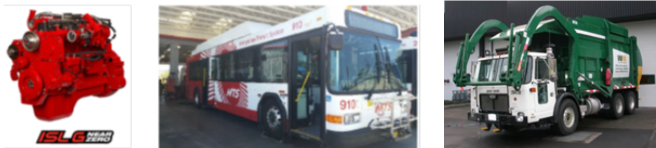
Figure 20. Cummins Westport 8.9 Liter ISLG near zero natural gas SI engine (left); Examples of a bus and refuse truck that rely on natural gas (center and right) SOURCE: Cummins Westport presentation, Fuels and Transportation Merit Review, CEC, December 2, 2015
