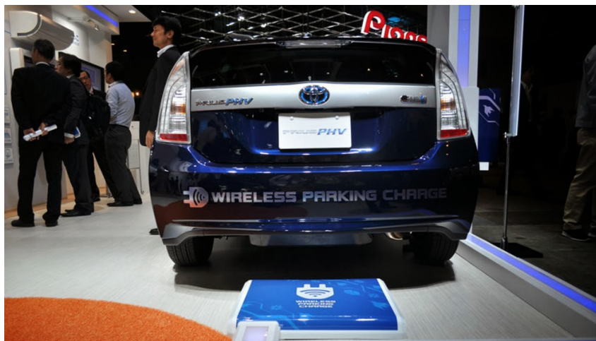
Figure 5. WiTricity wireless power transfer systems
