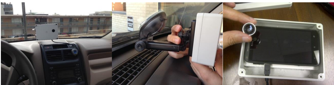
Figure 3. The far left photo shows a front aspect photo of the final N-DAD device. The center photo shows the mounting device used to secure the N-DAD devices onto participants' car windshields. The far right photo shows the positioning of the smartphone within the housing.
