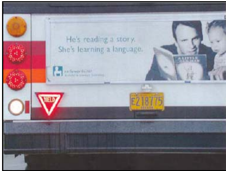
Figure 19 Tri-Met LED Yield sign (Source: TCRP Synthesis 49)
