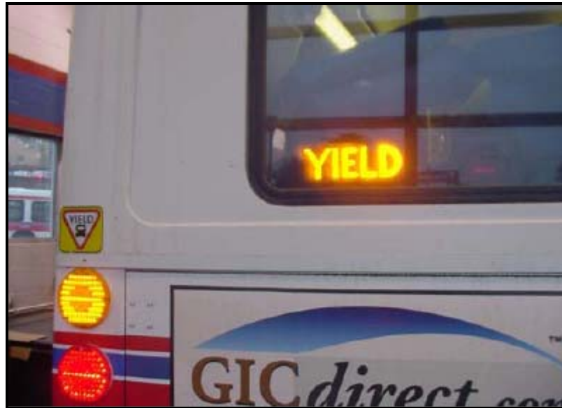
Figure 18 British Columbia Transit YTB decal and Yield LED Sign (Source: TCRP Synthesis 49)
