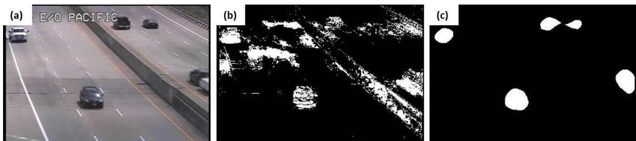
Figure 3.2 Advantage gained by using MHI: (a) original image, (b) GMM detection results, (c) MHI detection results
