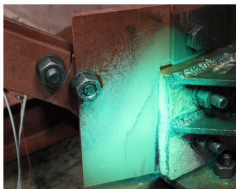
Figure 3-3: Cracks on 20-deg. skewed crossframe 775,000 cycles into Trial 2
