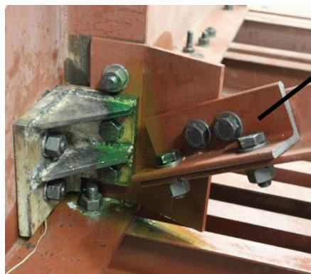
Figure 3-2: Crack on 20-deg. skewed crossframe 697,000 cycles into Trial 20-2, and the bolted steel angle used to repair it
