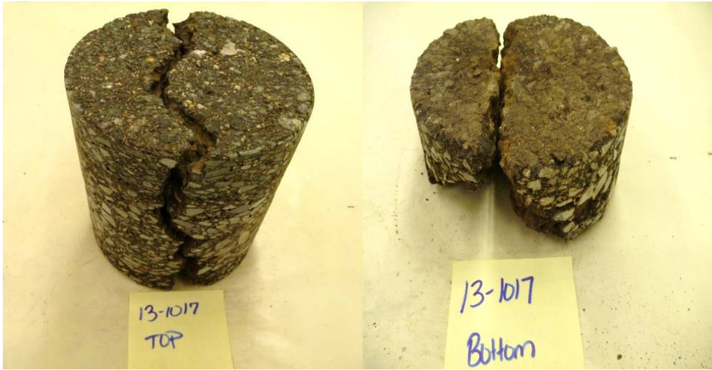
Figure 9. Full depth Crack Seen in Site F, SR 24 in Appomattox County
