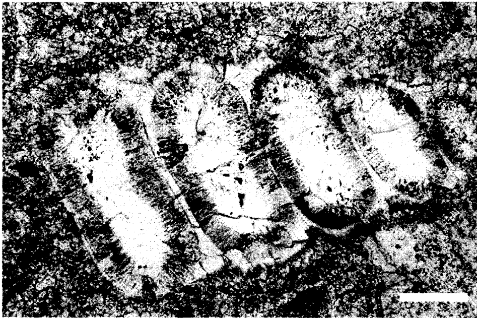
Figure 2.8 Photomicrograph of gastropod mold lined with early fibrous cement that is overprinted by neomorphic calcite. Original micritic matrix is recrystallized to microspar and some pseudospar. (Sample RW-9; transmitted light; scale bar = 400 micrometers)
