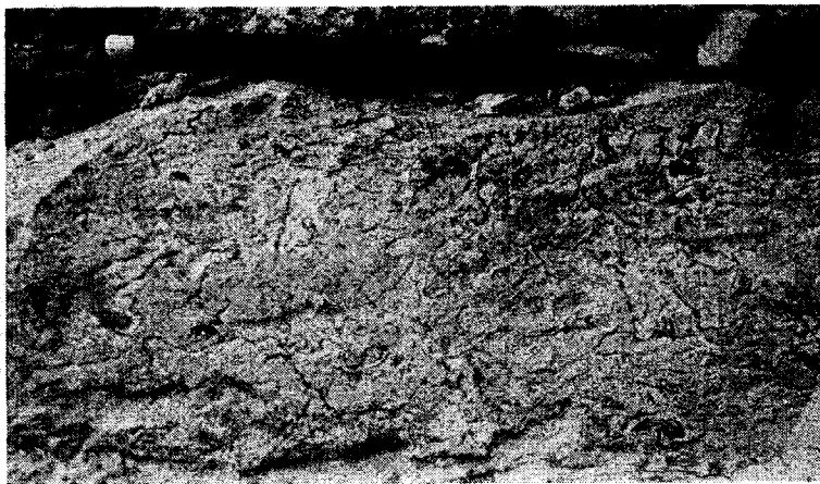
Figure 3.5. Photo of a bed of phylloid algal wackestone with completely disseminated argillaceous material throughout its thickness. This form of clay is recognized by the bluish-gray color it imparts to the rock. Due to the disseminated nature of the clay, it will become part of the aggregate following crushing of the rock.
