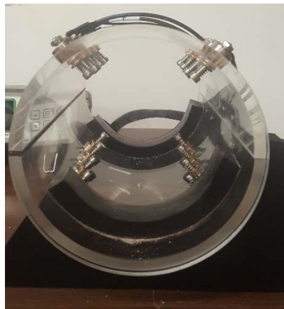
Figure 3.3 Surface electrical resistivity sample holder
