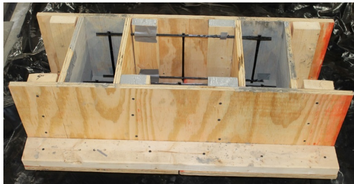
Figure 11. Typical Formwork for Development Length Testing with NEFMAC
