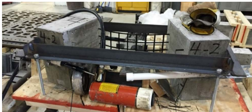
Figure 14. Typical Failure of a Development Length Specimen
