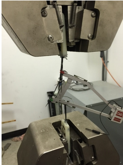
Figure 8. Typical Failure of Tensile Specimen
