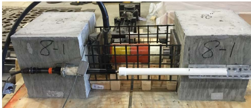
Figure 12. Typical C-Grid Test Set Up
