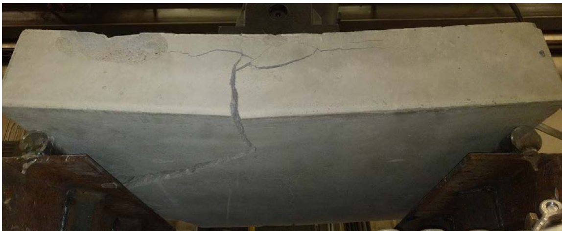
Figure 4.16 Crack \frac{3}{4} inch wide, (36,000 cycles)
