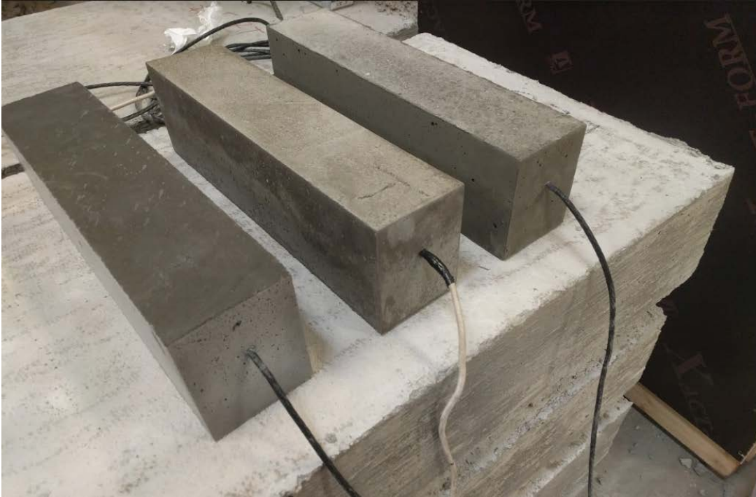
Figure 2.8 Embedded Litz wire segments
