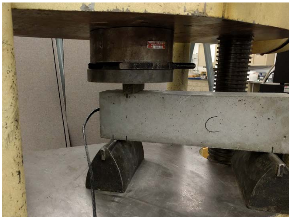
Figure 2.9 Break test set-up
