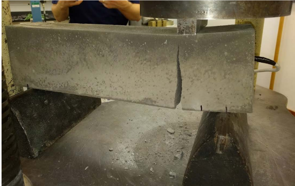
Figure 2.10 Concrete sample after failure
