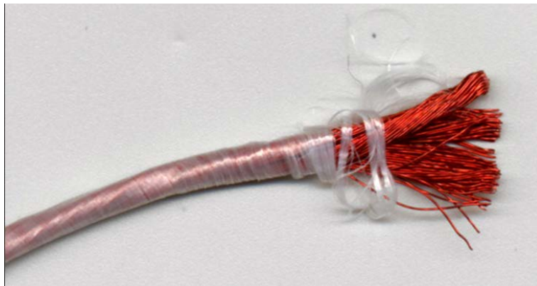
Figure 2.16 Litz wire with nylon sheathing
