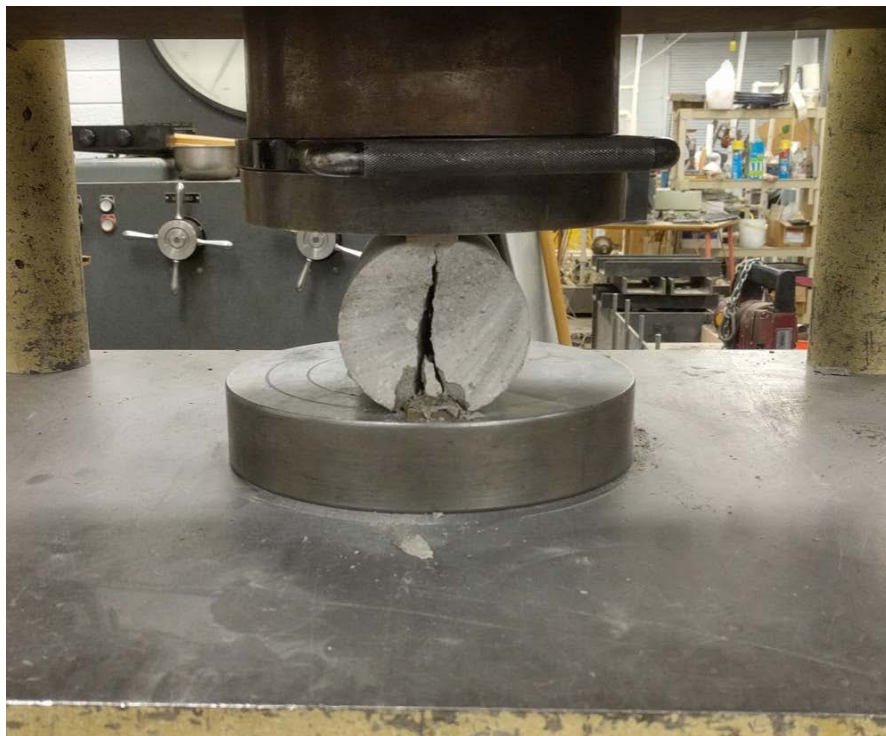
Figure 3.8 Split tension test
