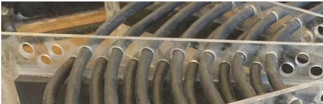
Figure 2.21 Close up of final pad vertically offset wire spacing
