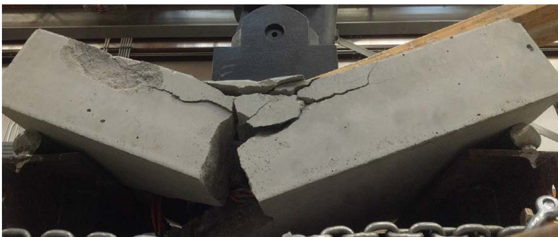
Figure 4.17 Failure (approximately 40,000 cycles)
