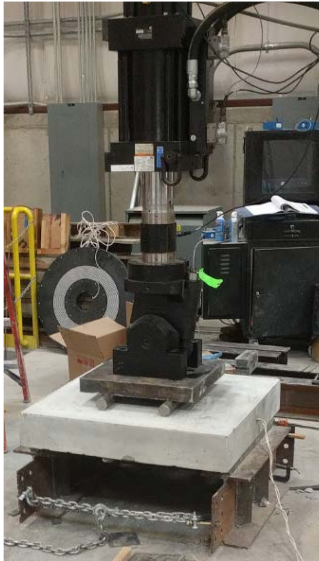
Figure 3.5 Four-point bending test set up
