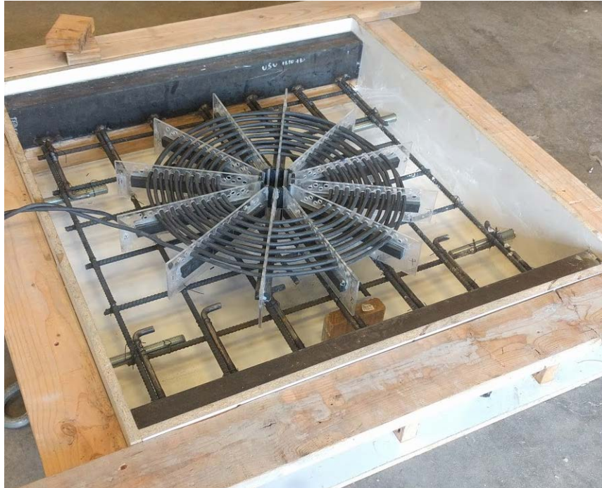
Figure 2.20 Final IPT embedment design
