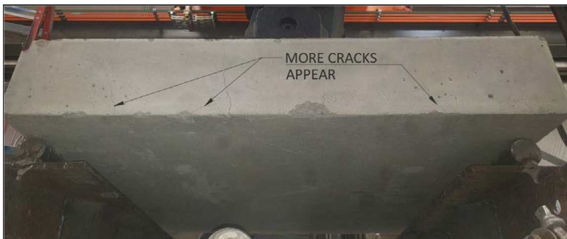
Figure 4.6 Load was increased to 9000 lbs. (approximately 20,000 cycles)
