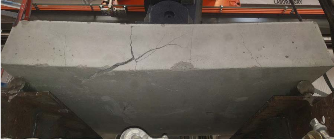
Figure 4.7 Cracks 1/2 inch (approximately 25,000 cycles)
