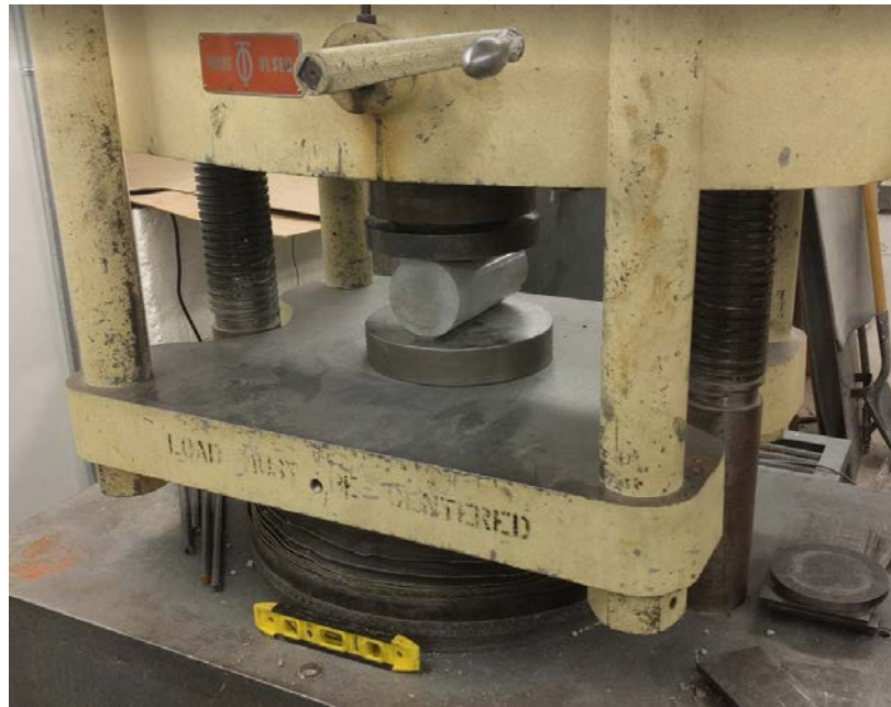
Figure 3.7 Split tension test set up
