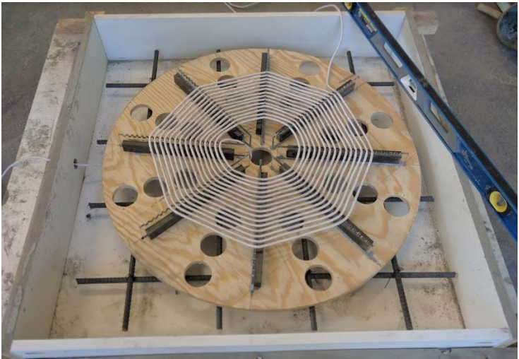
Figure 2.18 Test 3 IPT coil without aluminum plate
