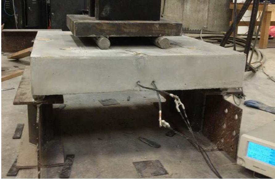
Figure 4.28 Other Sample tested with four-point bending test
