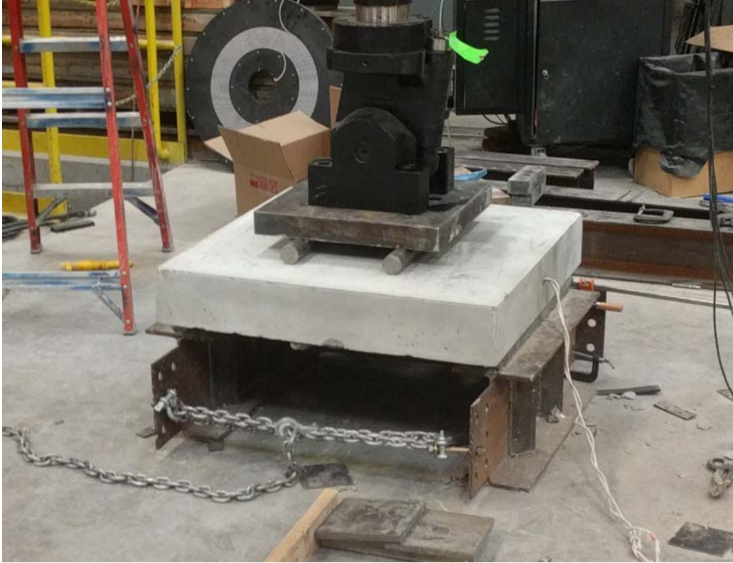
Figure 4.1 First fatigue test set-up
