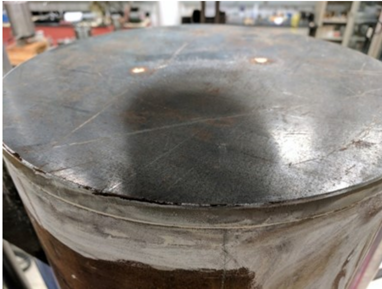
Figure 2.2 (a) Concrete cylinder with strain gages. (b) Composite pile within the load frame. (c) Steel plate on top of composite pile.
