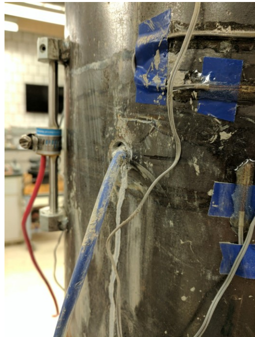
Figure B.2 (a) Vibrating wire strain gage. (b) Embedment hole on steel pile
