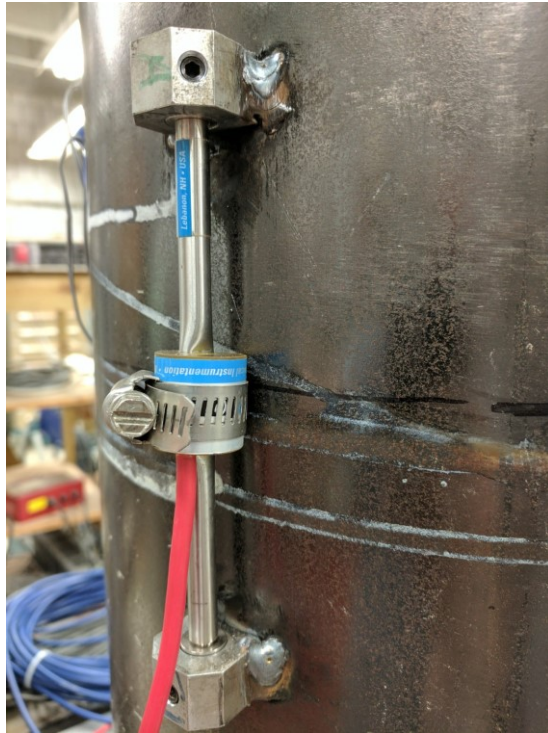
Figure B.5 Vibrating wire strain gage on pile surface
