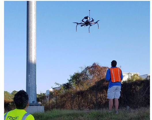
A researcher launches a small unmanned aerial vehicle for inspection of high mast light-pole.
