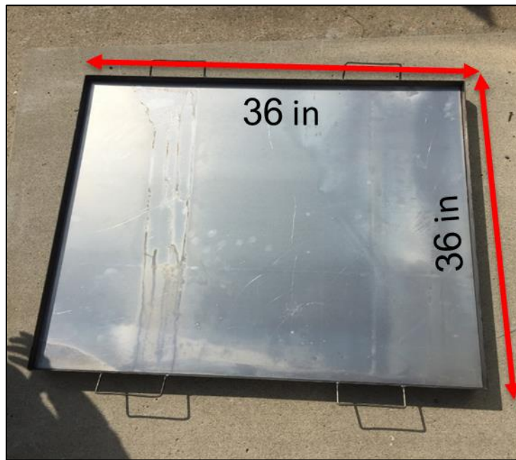
Figure 56. Square yard pan for conducting quality control measurement of aggregate application rates
