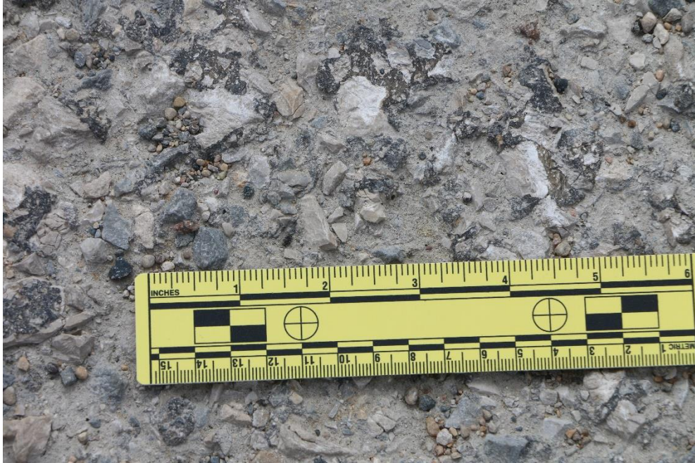
Figure 150. Appearance of Otta seal surface on a test section six months post construction, shown with scale
