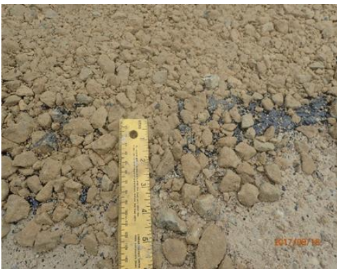
Figure 22. Aggregate used for Otta seal on CR 116, Winona County, Minnesota
