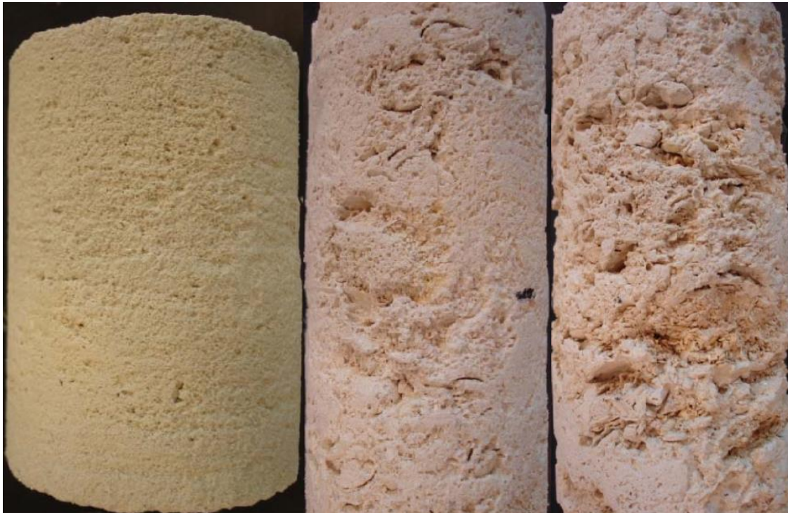
Figure 2.43 Different limestone surface textures (Sarno et al. 2010).
