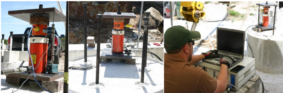
Figure 3.18 Pull-out load test in progress.
