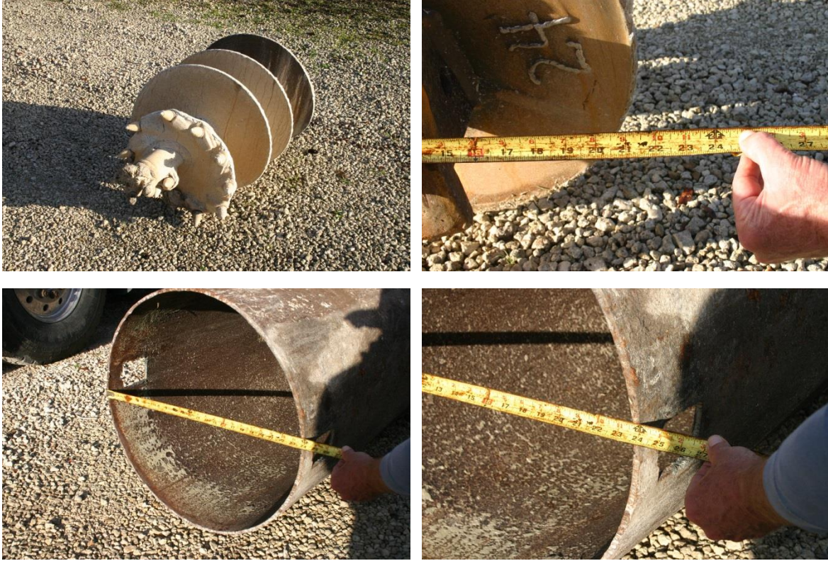
Figure 4.9 Rock auger and casing used to excavate both shafts.
