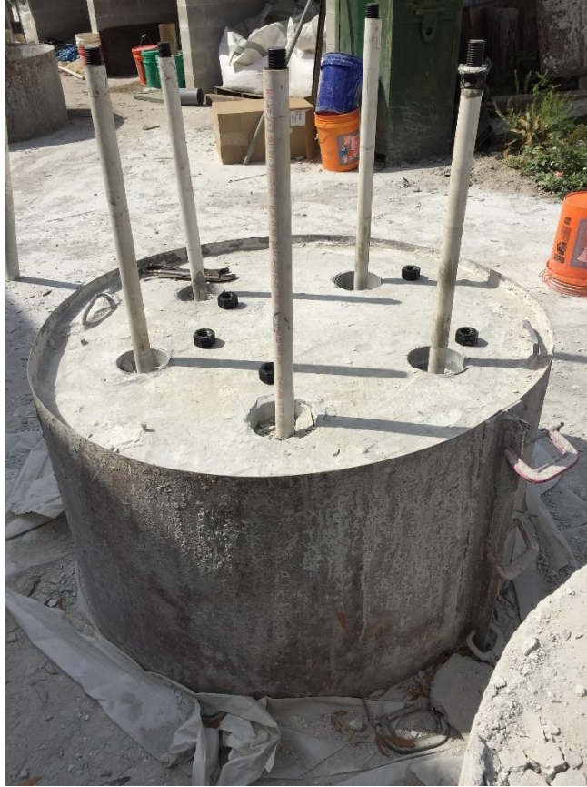
Figure 5.1 Rock socketed specimens being prepared for pull-out tests.
