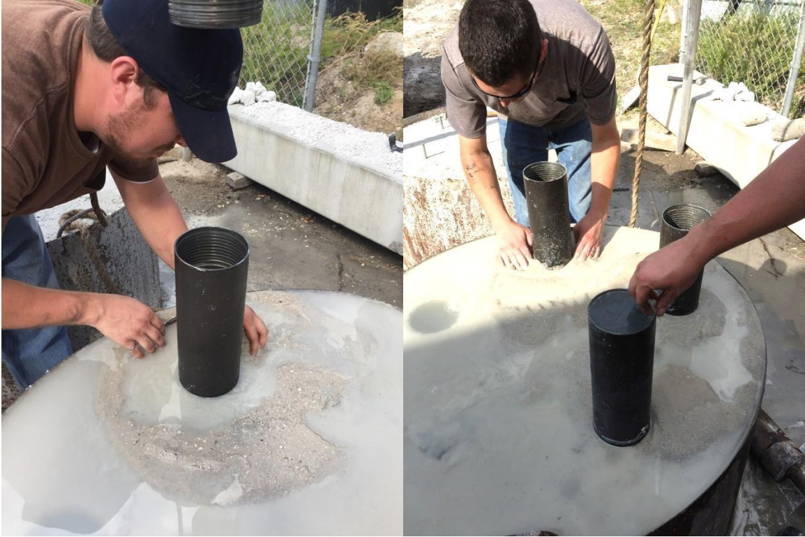
Figure 3.12 Cuttings replacement on the outer perimeter of the casings.
