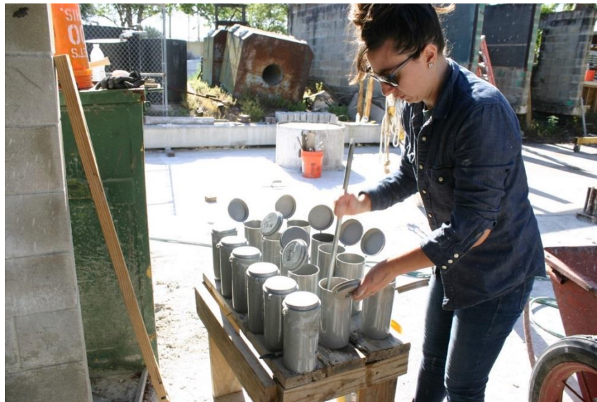
Figure 3.4 Preparation of cylinders from limestone bed material.
