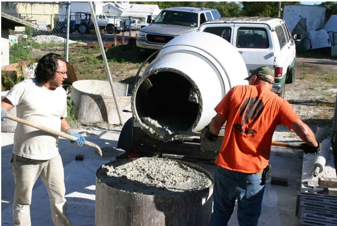
Figure 3.2 Casting of simulated limestone bed.
