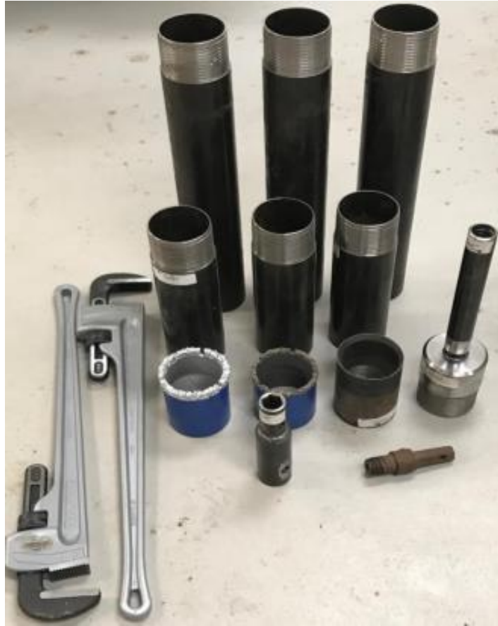
Figure 3.6 Casing cutting tips, drive shoe, casing extensions and drill rod couplers.
